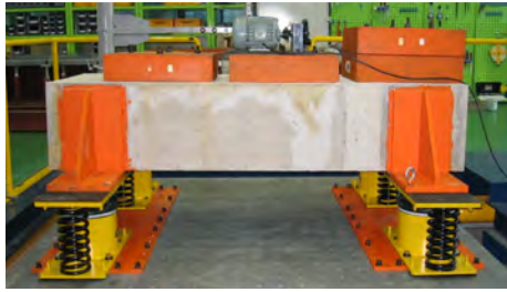
Fig. 2 EDG model with spring-damper units for the shaking table test
