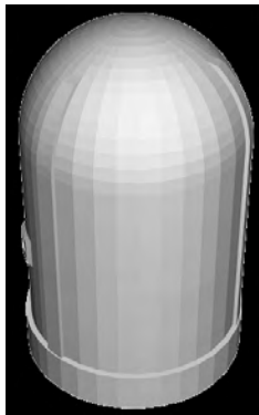
(a) 3-D FEM model (b) Fundamental mode shape (c) Lumped Mass Model Fig. 2 3-D FE Model, Fundamental Mode Shape and Lumped Mass Model of the Containment Building
