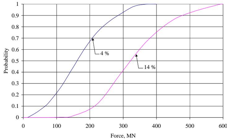
**Fig.3 Probability of Reinforcing Bar Failure in the Initial Tension Side of the Impacted Wall for Failure Strains of 4 and 14 percent**
