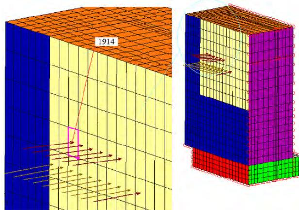
**Fig. 1 Finite Element Model of the Ignalina NPP Building**
