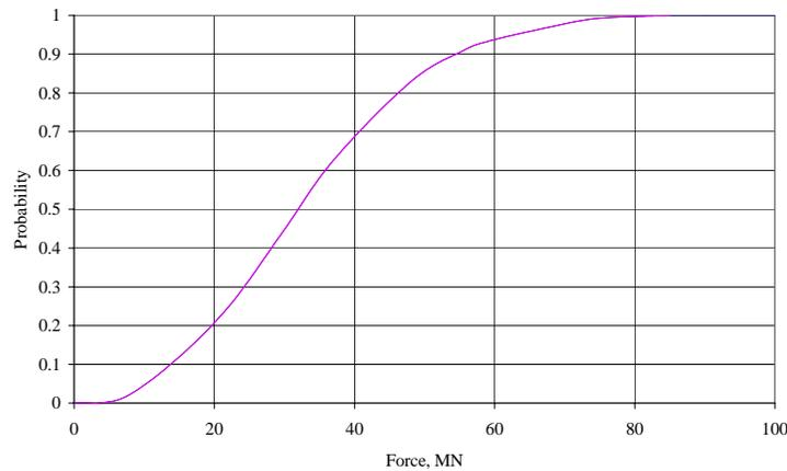
**Fig. 2 Probability of a crack developing in the initial tension side of the impacted wall**
