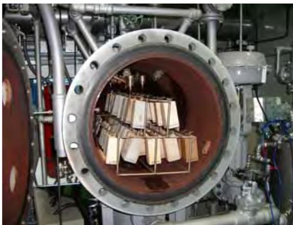
Fig. 9 : Autoclave for the DBA Test
