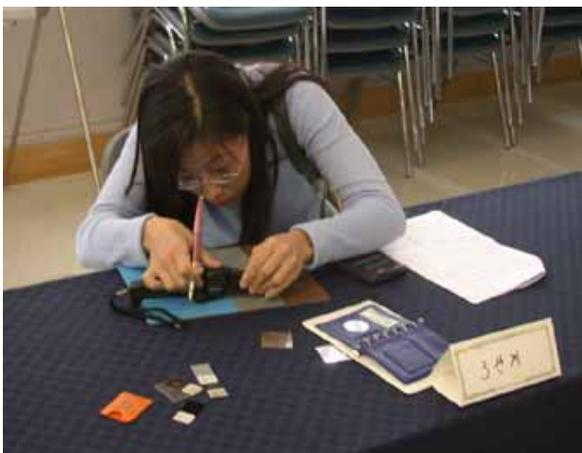
Fig. 3 : Measurement of Coating Dry Film Thickness
