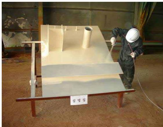
Fig 6. : Coating Applicator's Exam. for Steel Surfaces
