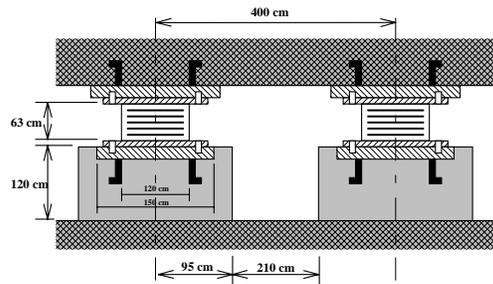
**Fig. 4 Installation Concept of the Isolators**
