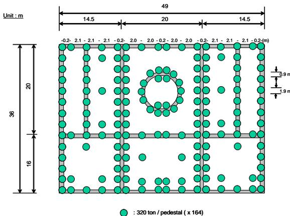
**Fig. 3 Schematic Arrangement of the Isolators**
