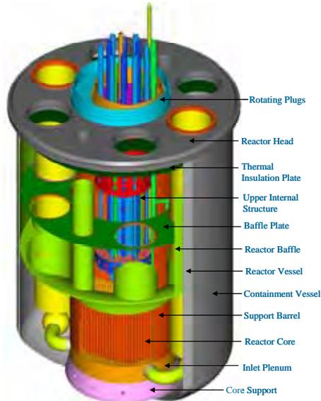
**Fig. 2 Reactor Internal Configuration**
