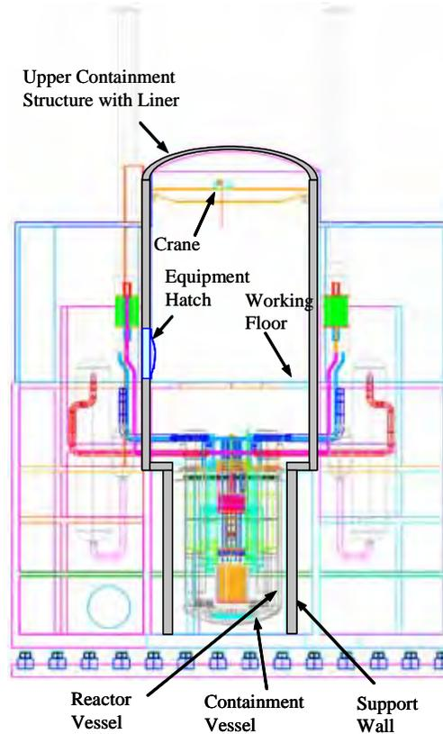
**Fig. 6 Schematic Drawing of the Containment Concept**
