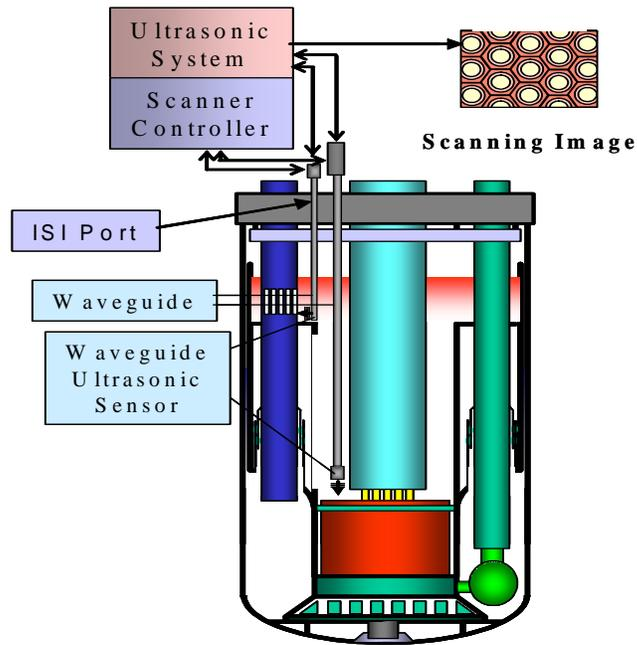
**Fig. 7 Visual Inspection Concept Using the Ultrasonic Waveguide Sensor**
