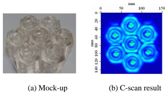
**Fig. 8 Visualization Images of the Reactor Core Mock-Up**
