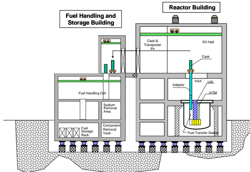
**Fig. 5 Arrangement of the Reactor Refueling System (RRS)**
