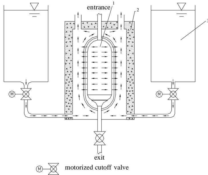
Figure 6 Sketch of water flow and heat transfer in pebble catcher
