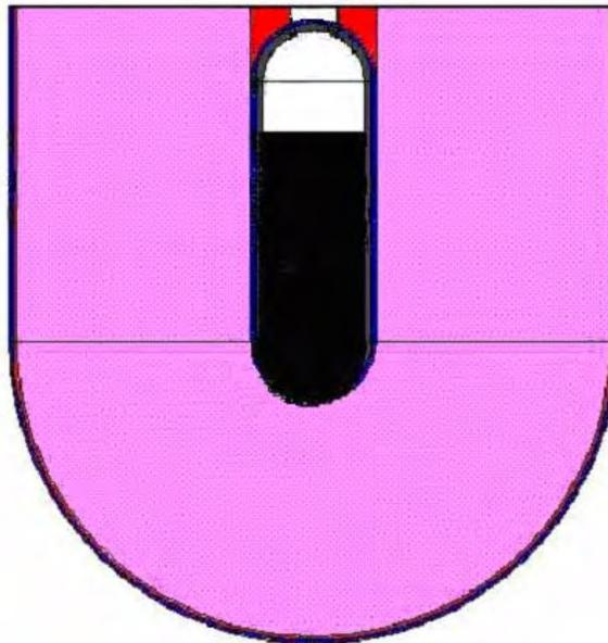
Figure 4 Criticality safety calculation model with packing densities 0.74 and water layer thickness 3000mm
