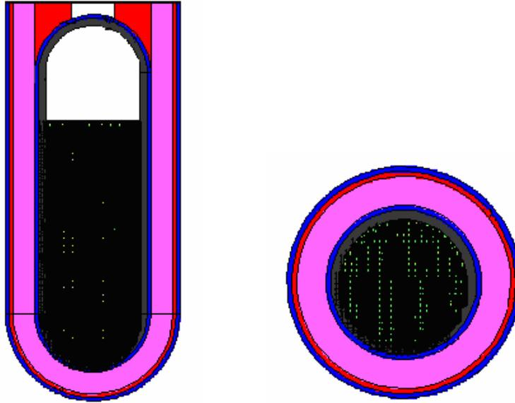
Figure 3 Criticality safety calculation model with packing densities 0.61 and 0.74, respectively, water layer thickness 300mm
