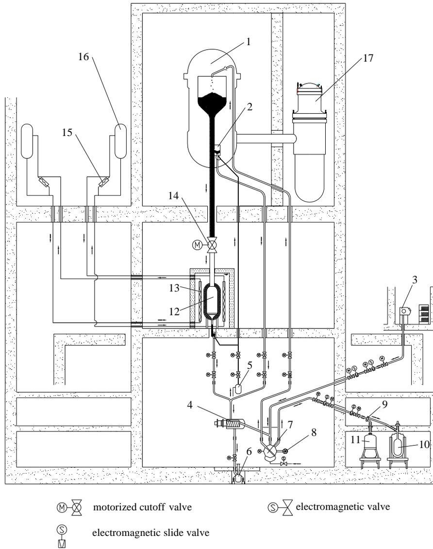
Figure 1 layout of a 50 MW pebble bed reactor with a fast pebble discharge system
