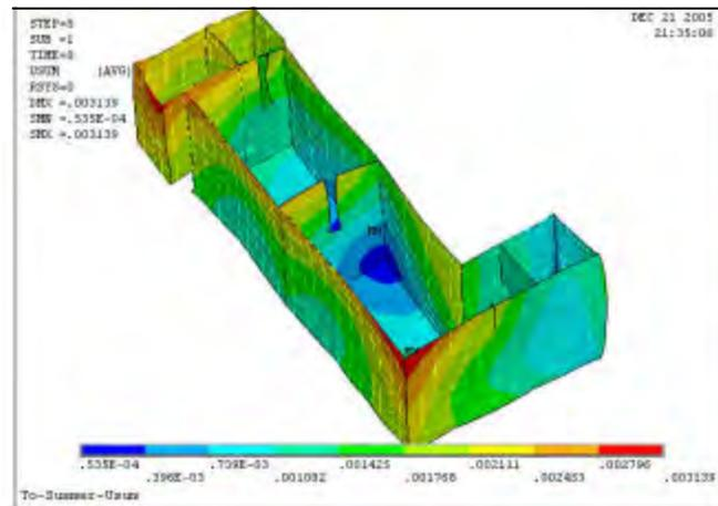
**Figure 5 - Deformed shape of SSSB pool under Thermal loading**
