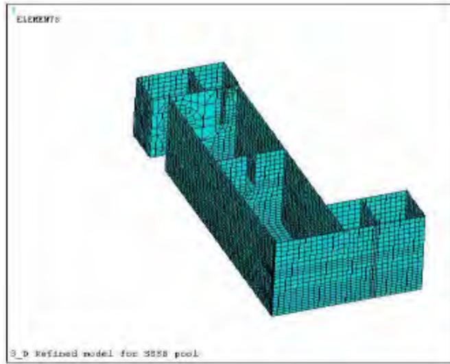
Figure 2 - 3-D FE Model of SSSB Pool
