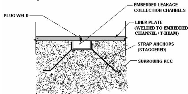
Figure 1 - Components of Liner System
