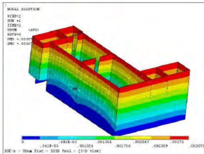
Figure 4 - Deformed shape of SSSB pool under Seismic load (SSE NS)
