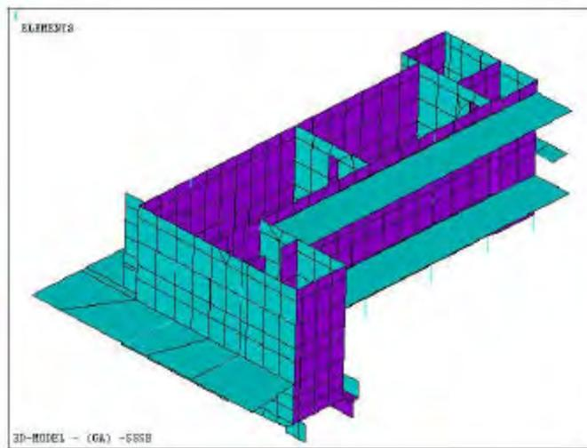
Figure 3 - General Arrangement of SSSB Pool (with surrounding concrete slabs and base columns)
