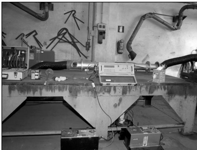
Fig. 4 The cutting workshop: close up with the measurement chimney, the probe for the feeding of the filters and various instrumentation.
