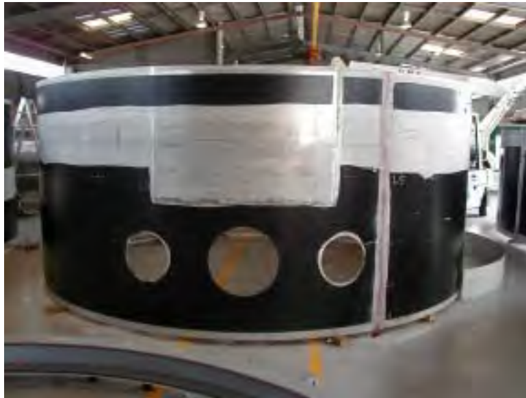
Figure 18 – Rolled and welded sheet
