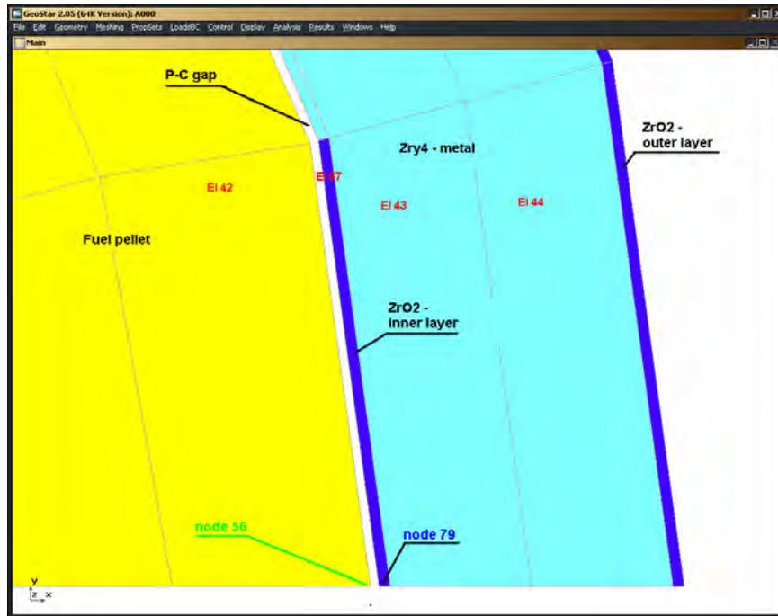
Fig. 8 Nodes No. 56 and No. 79, where the effective stress is demonstrated
