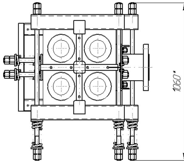
Figure 6 – Tested core of TKR-F (graphite) rig with four graphite blocks (top view)
