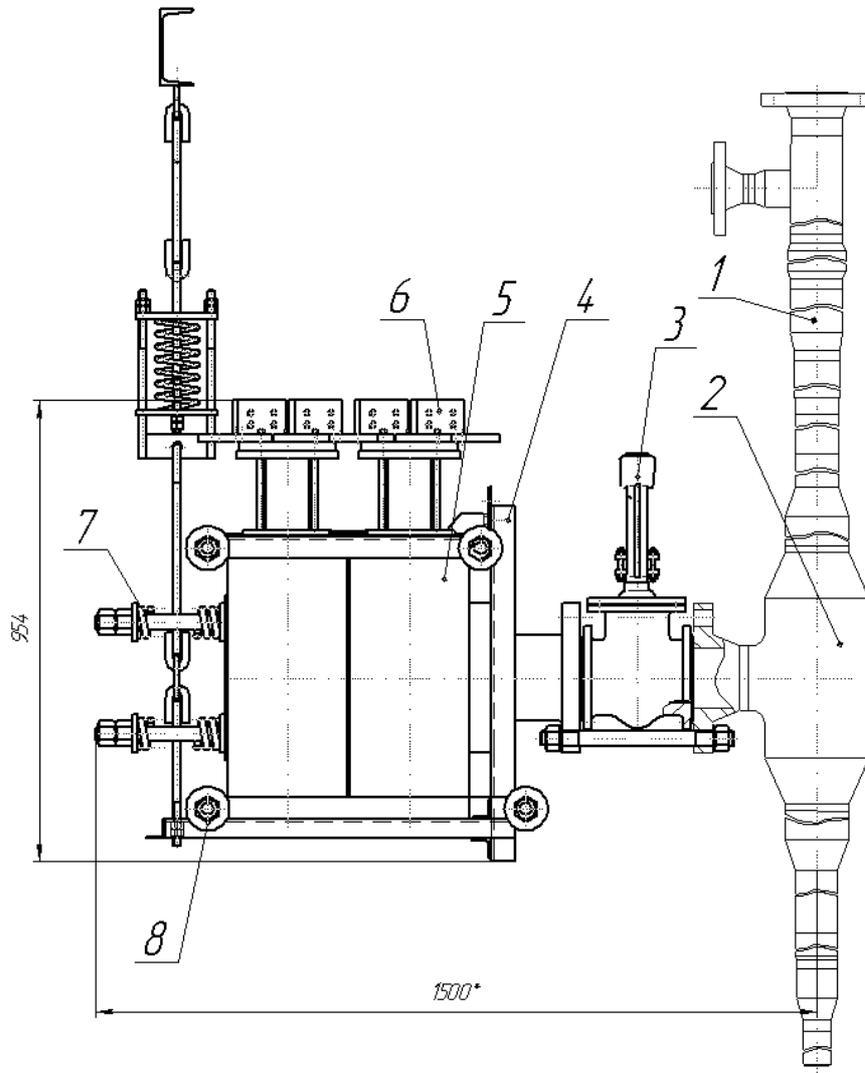
1 – steel tube; 2 – T-bent; 3 – valve; 4 – attachment point for blocks; 5 – graphite blocks; 6 – heater; 7 – longitudinal springs; 8 – lateral springs.
