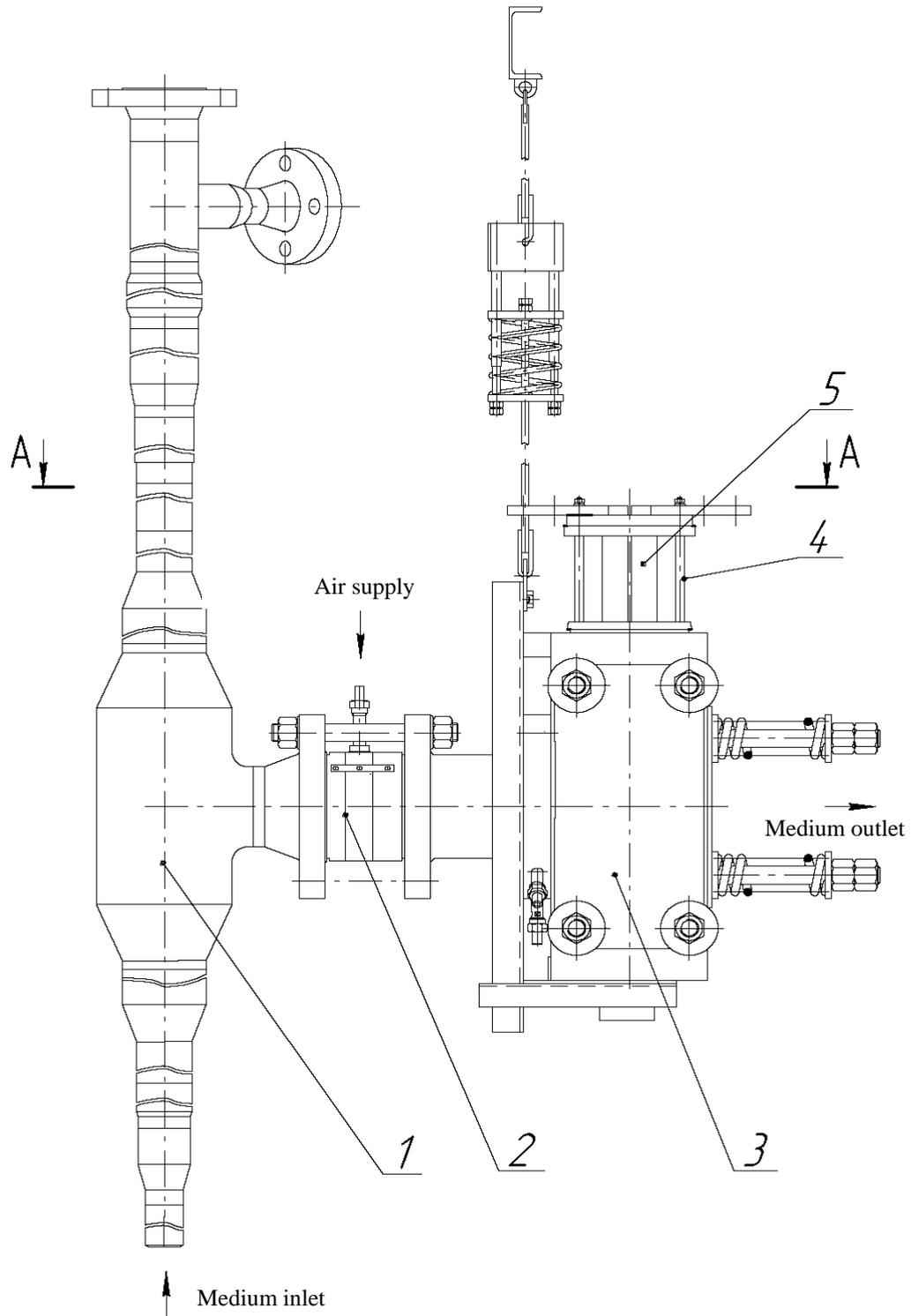
1 – T-bend; 2 – membrane unit; 3 – graphite block; 4 – fitting of the heater; 5 – heaters;
