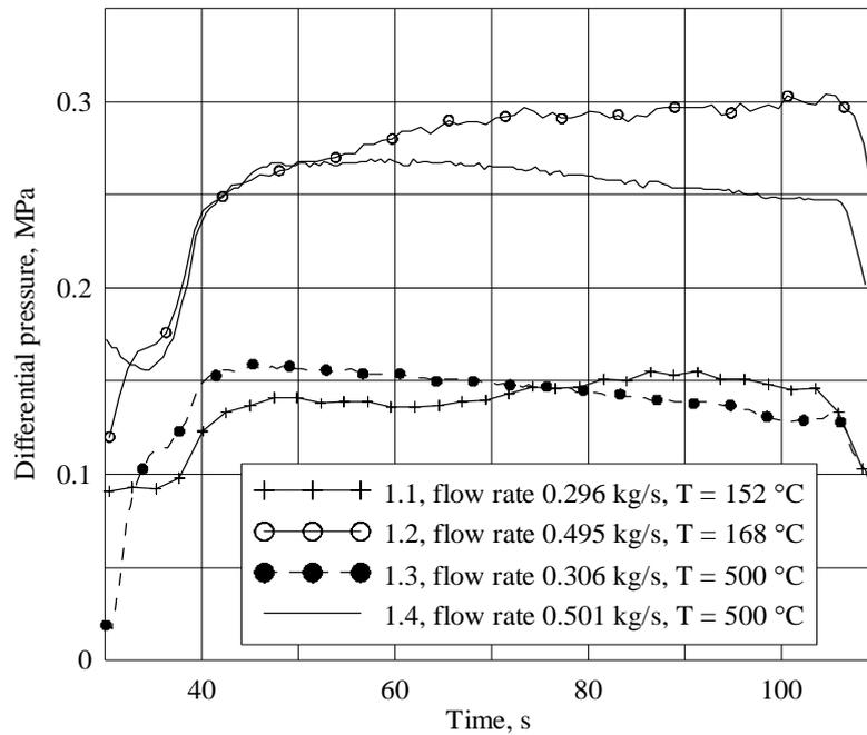
Figure 9 – Dependence of differential pressure along the gap on steam flow rate and graphite temperature
