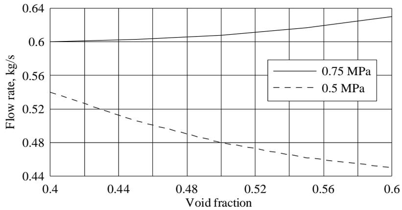
Figure 4 – Relation of maximum flow rate to void fraction at constant pressure 0.5 and 0.75 MPa
