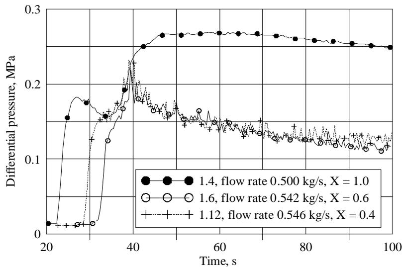
*Figure 10 – Dependence of differential pressure along the gap on steam-water mixture flow rate and void fraction X*
