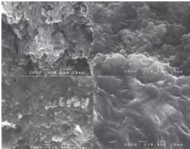
Fig. 2 Microstructure of the coated layers : (top-left) buffer (top-right) inner carbon (bottom-left) outer carbon (bottom-right) silicon carbide layer
