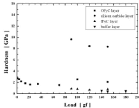
Fig. 3 Micro-hardness changes with load determined by nano-indentor
