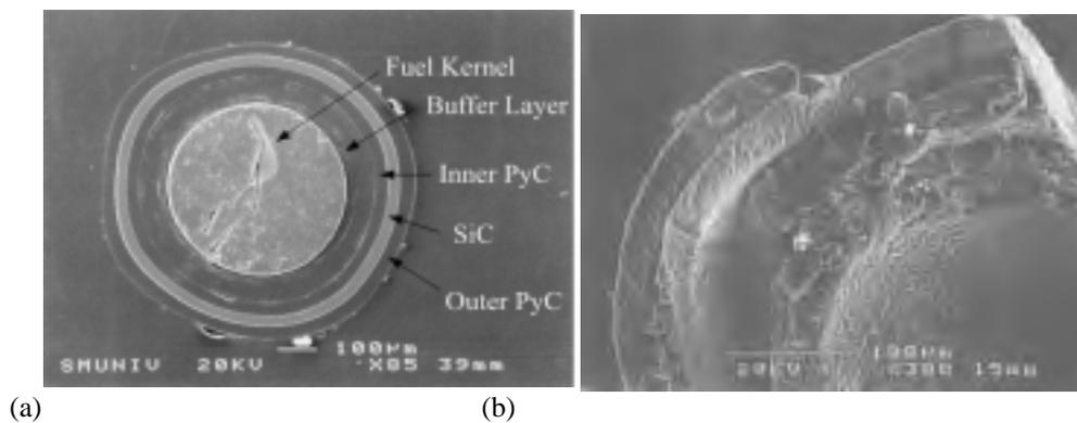
Fig. 1 Microstructure of the coated fuel : (a) cross sectional view of fuel (b) coated layers
