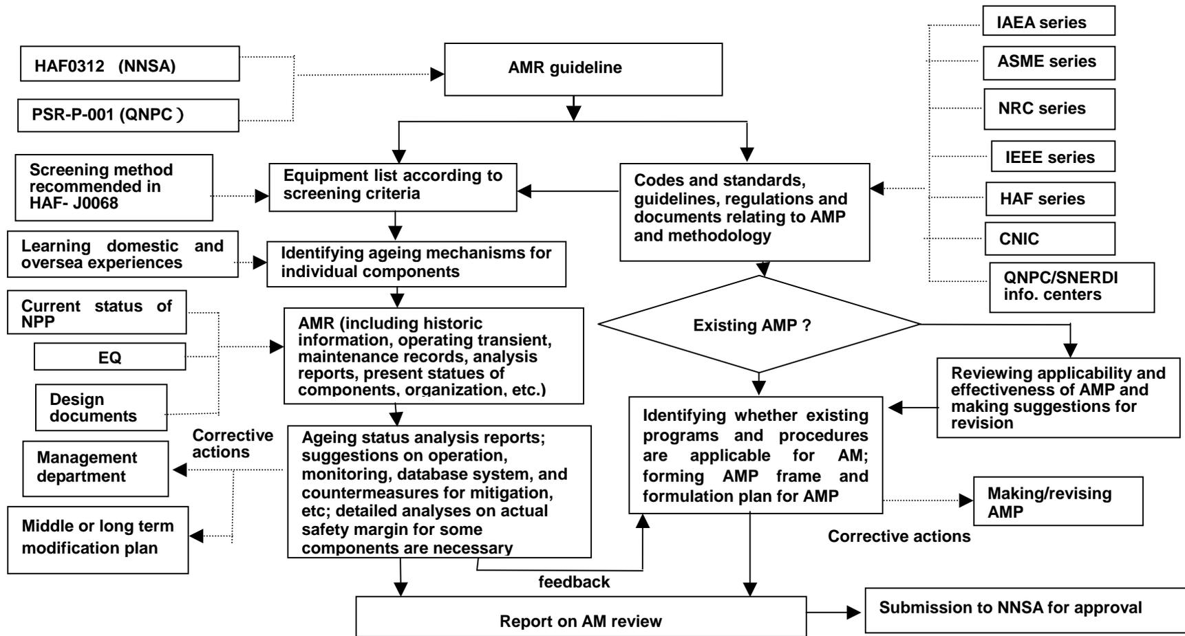
Figure 1 Procedure of AMR as part of PSR
