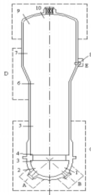
Figure 2 Fatigue evaluation sections for RPV
