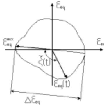
Fig.1. Determination of maximum strain equivalent range.
