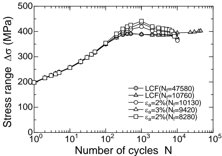
Figure 5. Variations of stress range in fatigue tests of 0.5 % strain range.
