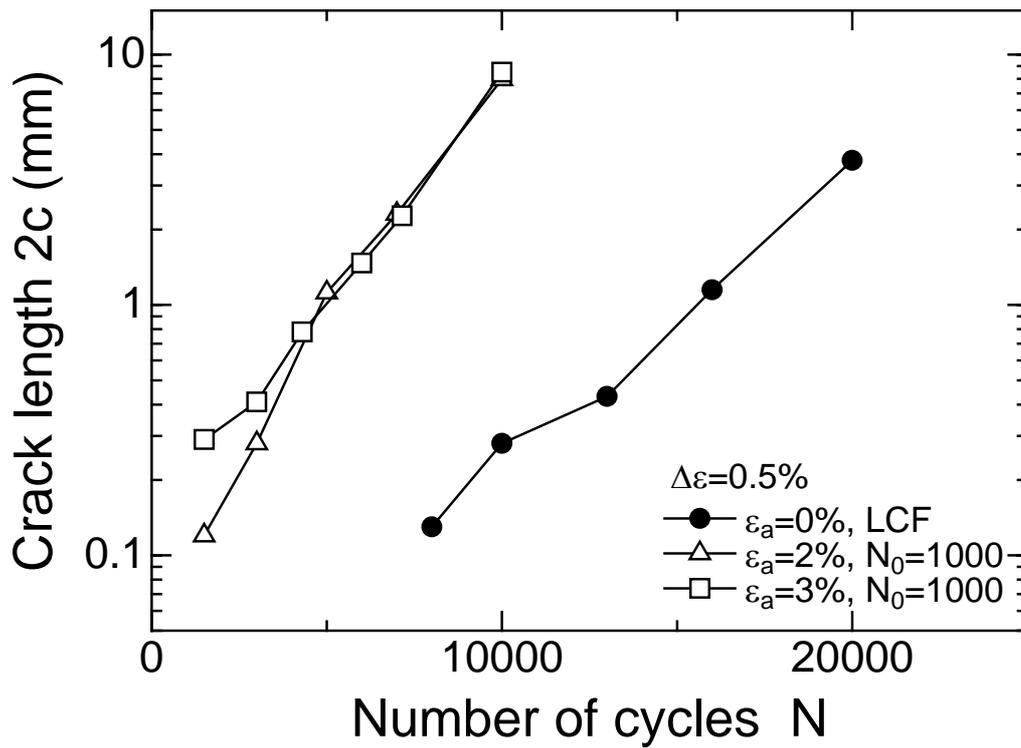
Figure 11. Micro-crack growth behavior observed in low-cycle and ratcheting fatigue tests of 0.5 % strain range.
