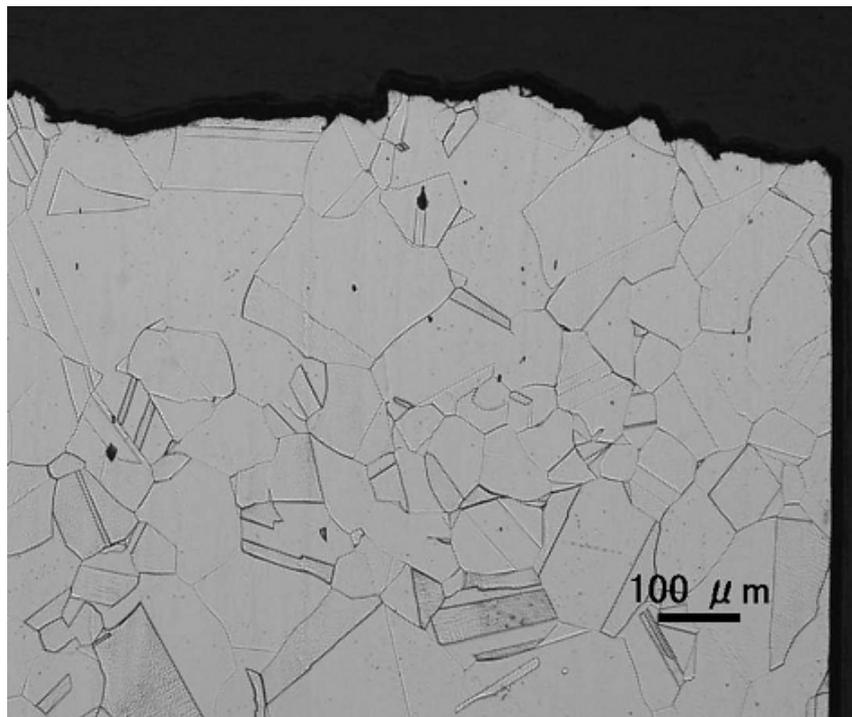
*(b) Ratcheting fatigue test of 3 % accumulated strain (failure life: 9420)*
