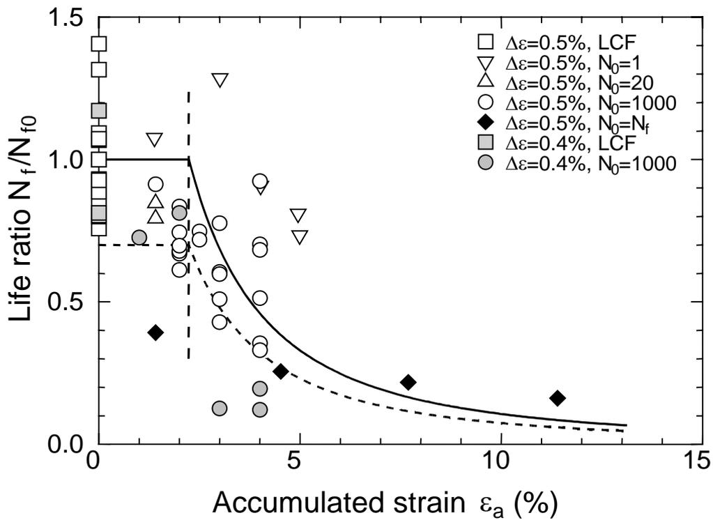
Figure 10. Relationship between life ratio and accumulated strain.
