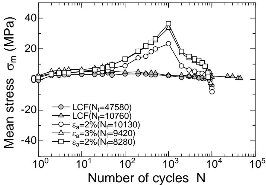
Figure 4. Variations of mean stress in fatigue tests of 0.5 % strain range.
