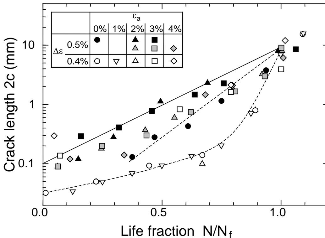
Figure 12. Relationship between crack length and life fraction.
