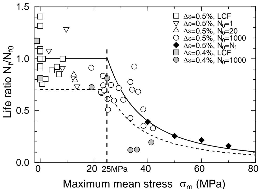
Figure 8. Relationship between life ratio and maximum stress range.
