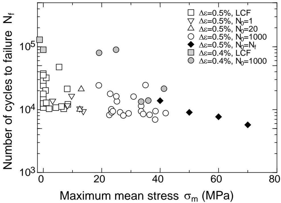
Figure 6. Relationship between failure life and maximum mean stress.
