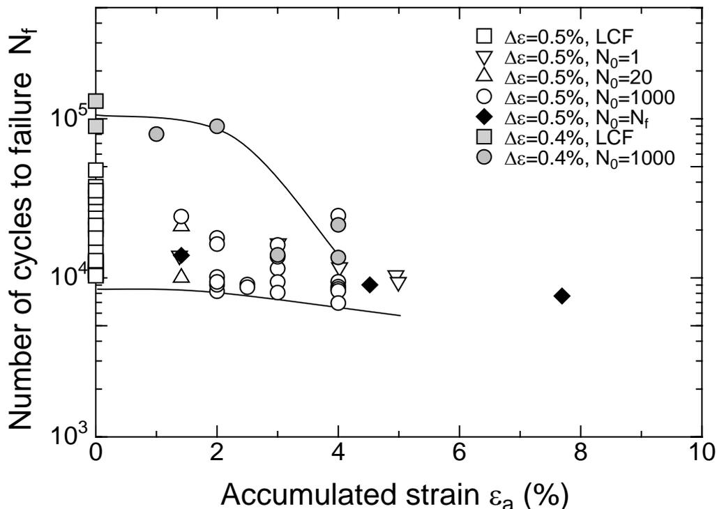
Figure 3. Relationship between failure life and accumulated strain.
