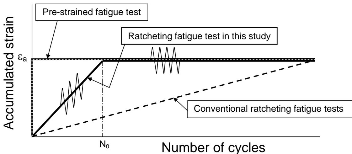
Figure 2. Outline of the ratcheting fatigue test in this study.
