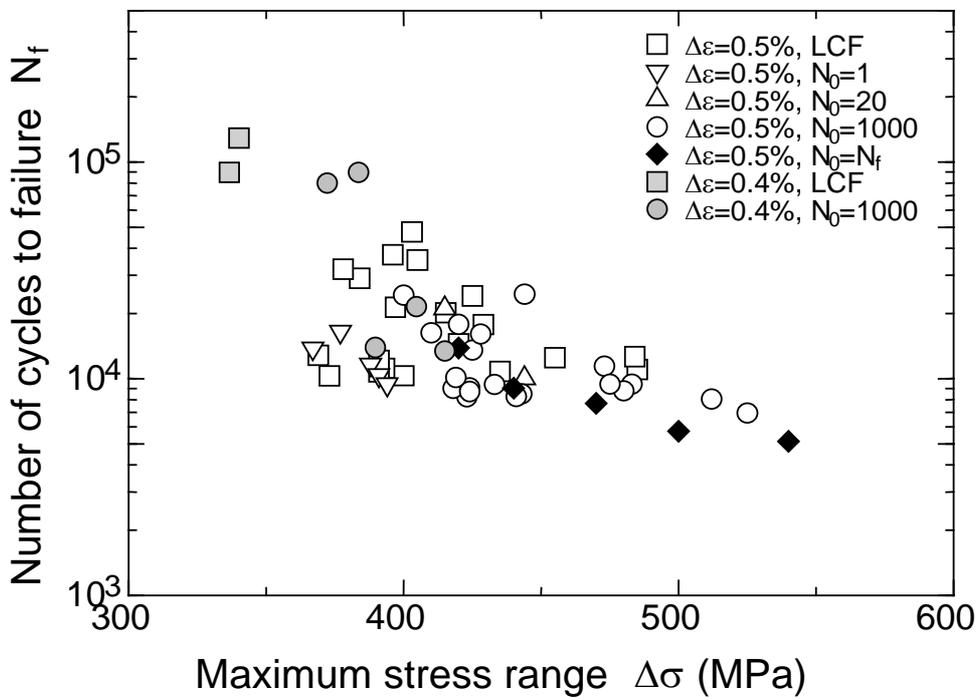
Figure 7. Relationship between failure life and maximum stress range.
