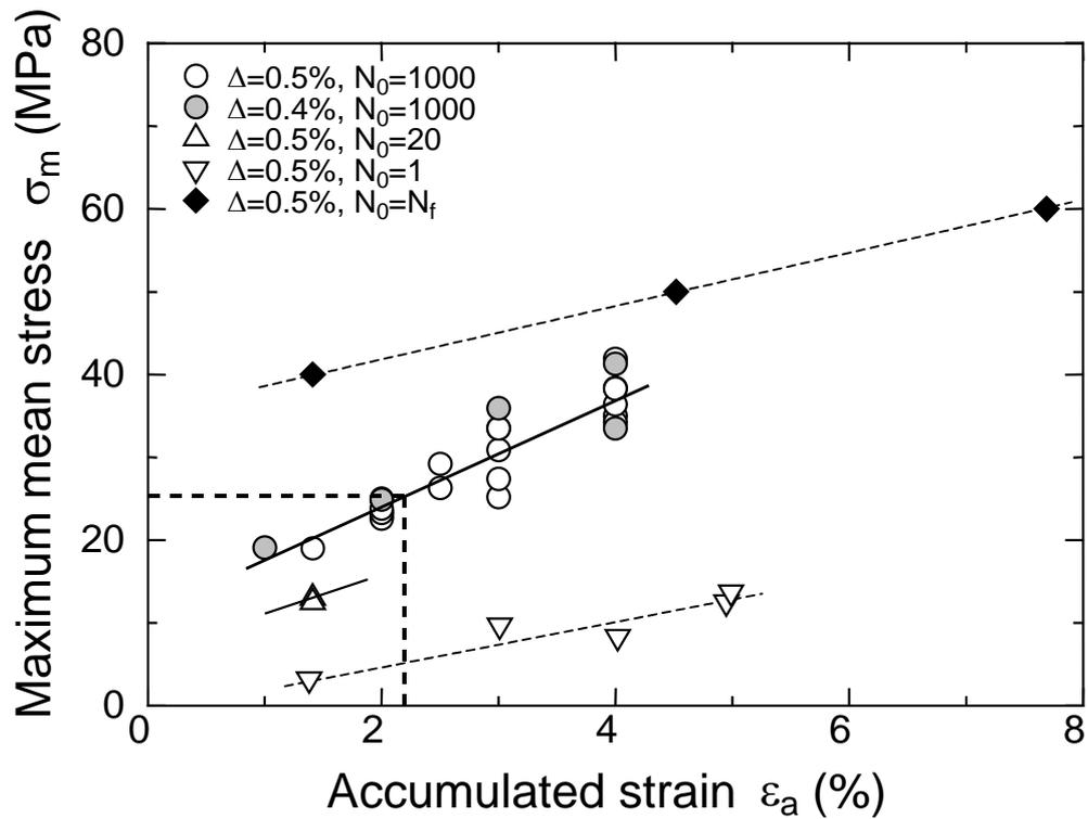
Figure 9. Relationship between maximum mean stress and accumulated strain.
