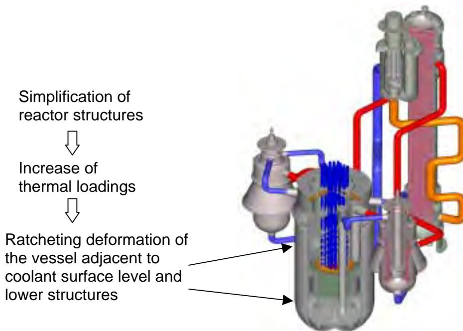
Figure 1. Schematic of commercialized fast Reactor.
