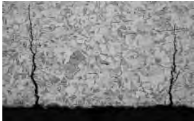
Figure 10 : Trans-granular crack propagation
