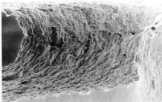
*Fig. 10: Blunting before onset of ductile tearing of the crack (acc. to Blumenauer)*
