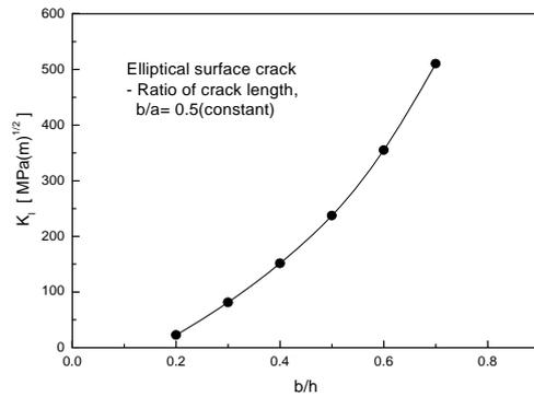
Fig. 6 SIF's according to  $b/h$  for a semi-elliptical surface crack in an elbow.
