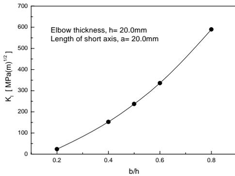
Fig. 5 SIF's according to  $b/h$  for a semi-elliptical crack in an elbow.
