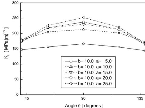
Fig. 3 SIF's according to angle of the crack tip for the surface crack in an elbow.
