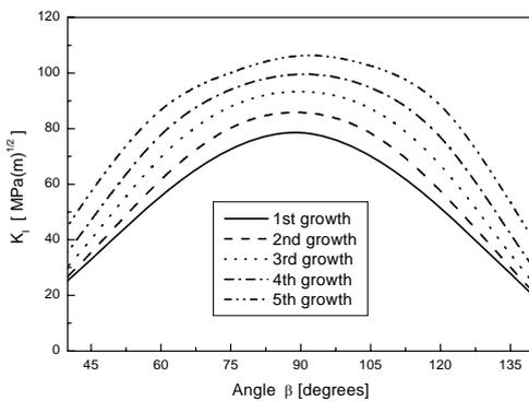
Fig. 7 SIF's of a semi-elliptical crack in an elbow under cyclic loading condition.
