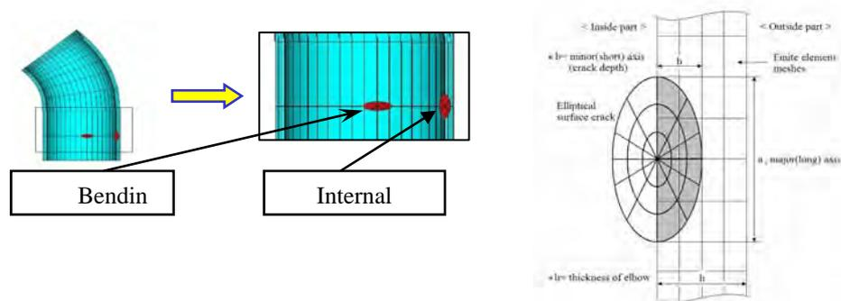
Fig. 2 Mesh configuration for a semi-elliptical surface crack in an elbow.
