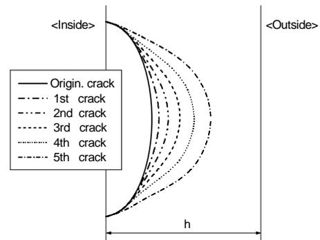
Fig. 8 Growth of an elliptical crack in an elbow under cyclic loading condition.
