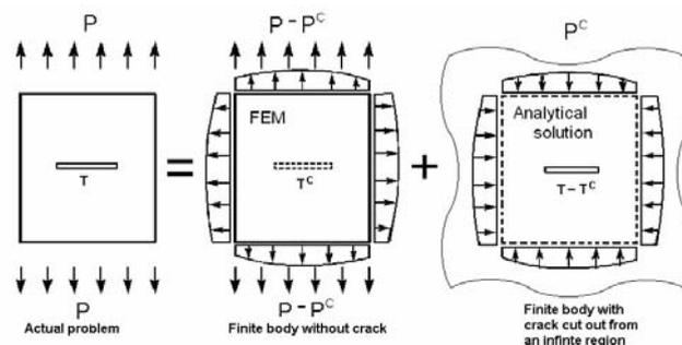
*Fig. 1. Superposition principle upon which the FEAM is based*
