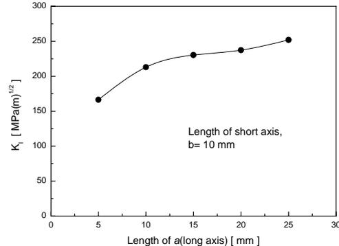
Fig. 4 SIF's according to the major length For a surface crack in an elbow.
