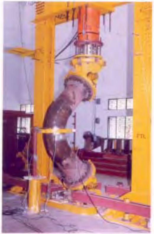
Fig. 1 Test Setup of Elbow with axial TWC at Crown (Seetharaman et al., 1999)
