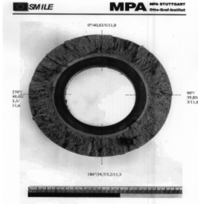
Fig. 6 - Brittle failure of the WP4 cylinder during final reloading
