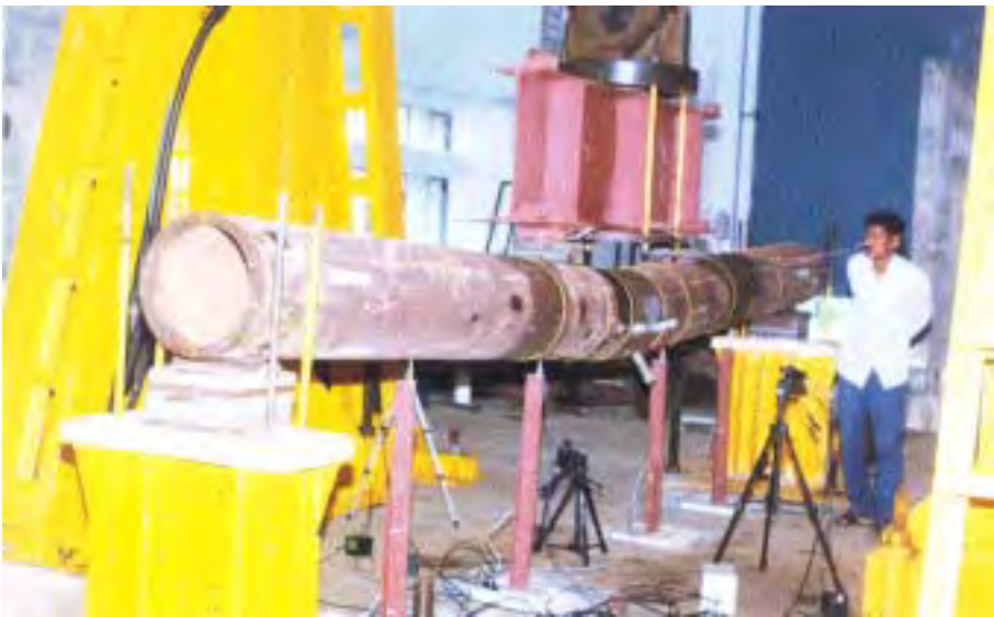
Fig. 4 Photograph of fracture test set-up of ferritic pipe under four point bending load
