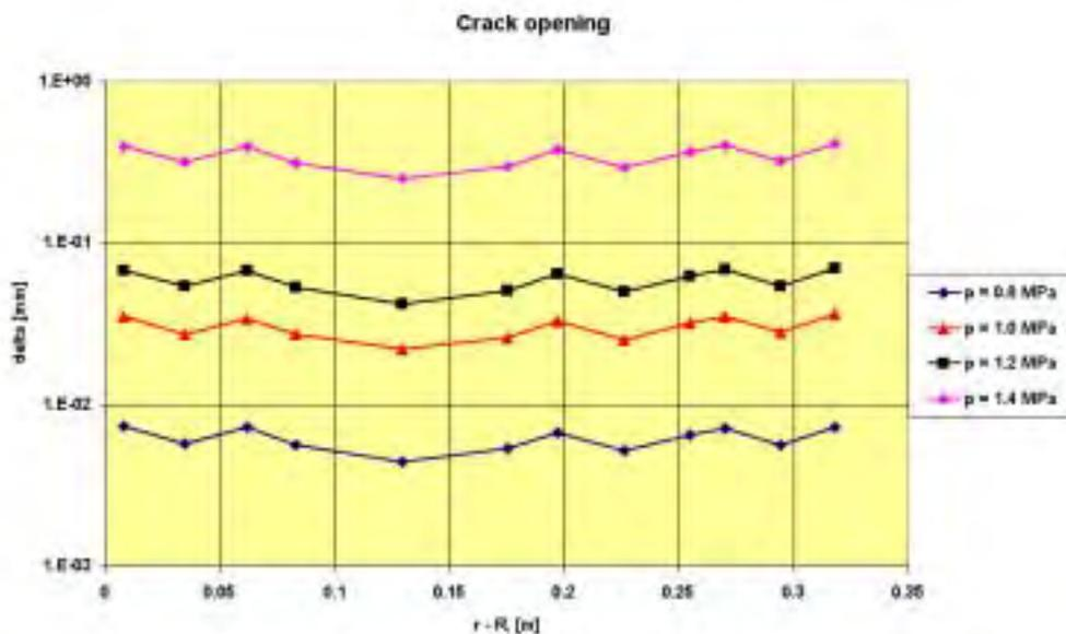
Fig. 22: Crack opening displacements for a line of integration points (in concrete) through the wall, slice model, pressure only case
