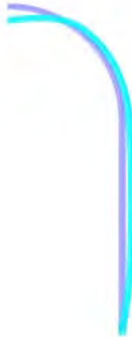
*Fig. 9: Deformation of axisymmetric model at 1.0 MPa (magnification of displacements = 50)*
