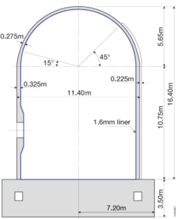
*Fig. 1: Major dimensions of the pre-stressed containment model (the wall includes hoop, meridional and radial rebars as well as hoop and meridional tendons)*
