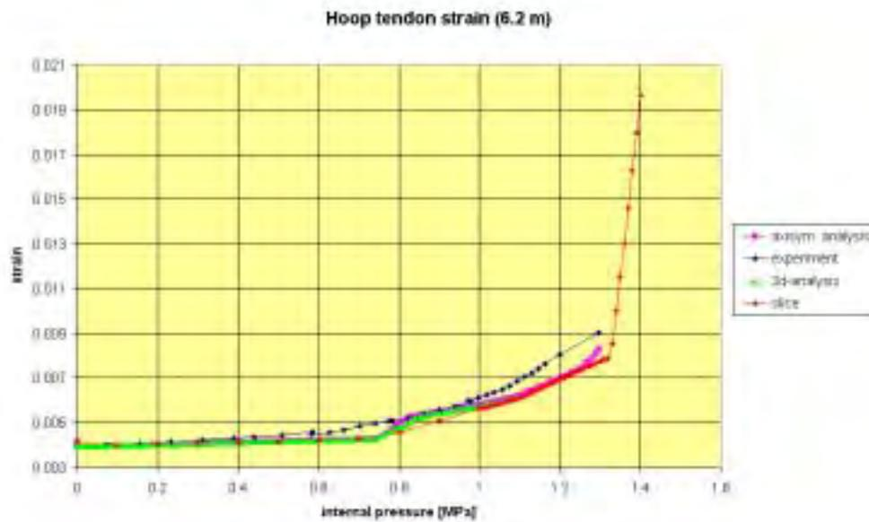
Fig. 15: Hoop tendon strains in the cylindrical part of the containment (position 6.2 m above basemat), pressure only – experimental values and calculated results
