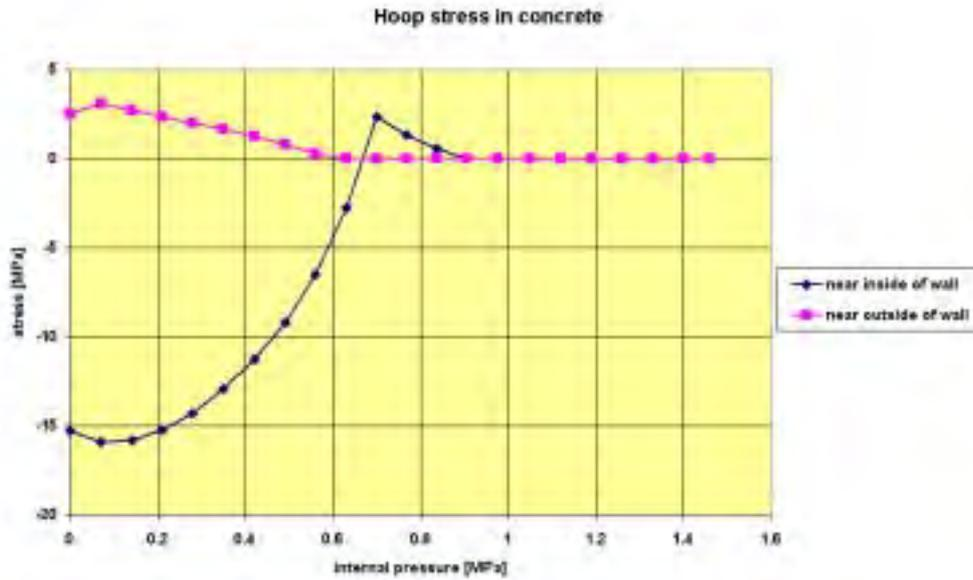
Fig. 18: Hoop stresses in the concrete for integration points near inner and outer wall, pressure only and temperature case 1 (slice model)
