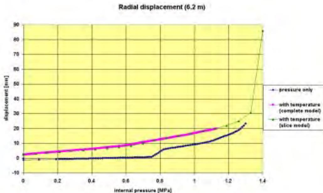
*Fig. 17: Radial displacement in the cylindrical part of the containment, pressure only and temperature case 1 (complete axisymmetric and slice model)*
