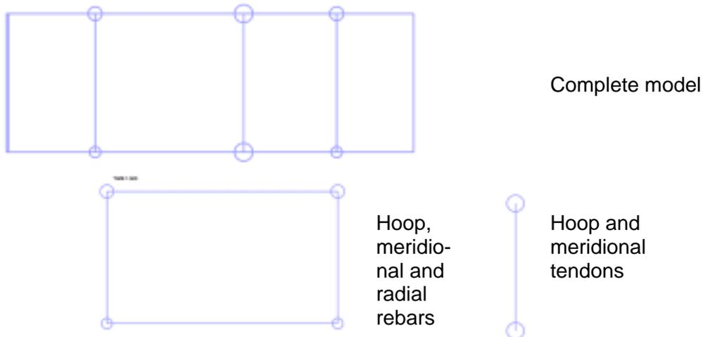
Fig. 5: Axisymmetric finite element model of a cylindrical section (slice model)
