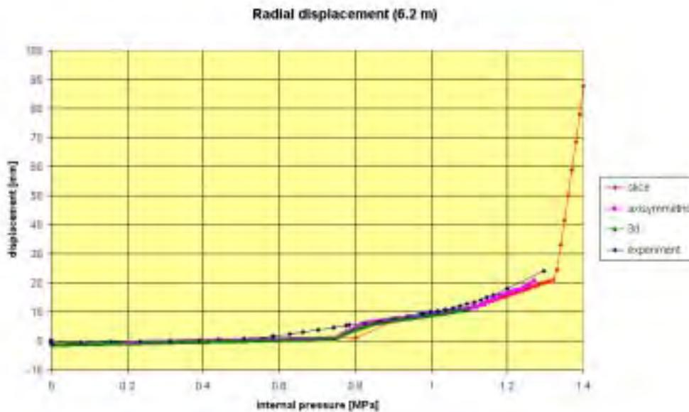
Fig. 12: Radial displacements in cylindrical containment part (position 6.2 m above basemat), pressure only – experimental values and calculated results
