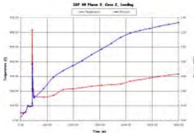
Fig. 7: Time functions for pressure and temperature at inner surface for ISP Phase 3, case 2 (from (Hessheimer, 2004))
