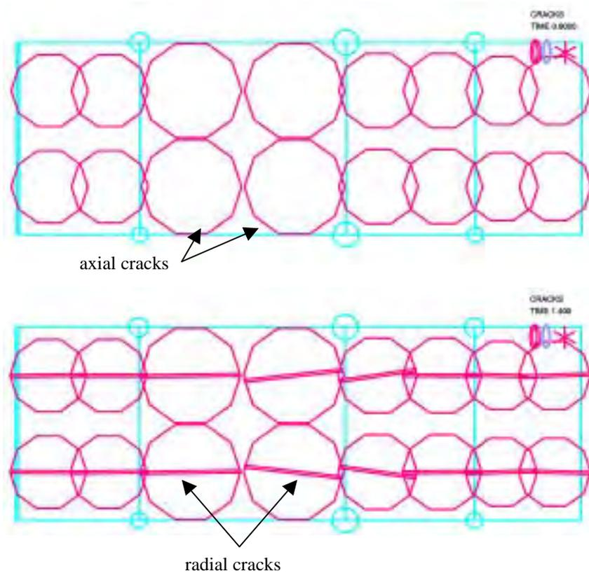
Fig. 16: Formation of axial and radial micro-cracks at internal pressures 0.8 and 1.4 MPa (axisymmetric slice model)
