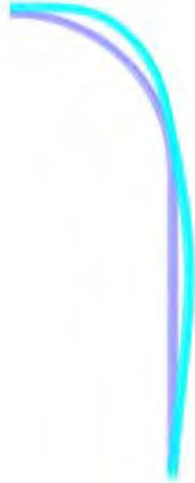
Fig. 11: Deformation of axisymmetric model at 1.4 MPa (only in calculation, magnification of displacements = 10)
