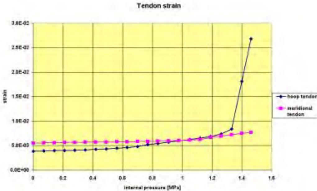
Fig. 19: Tendon strains (hoop and meridional), pressure only and temperature case 1 (slice model)
