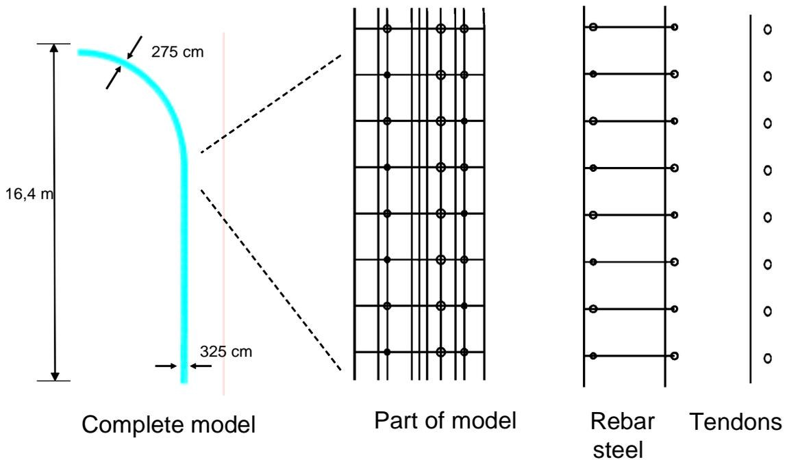
*Fig. 3: Axisymmetric finite element model*
