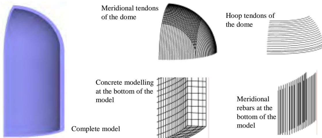
Fig. 4: 3d finite element model of a 90°-section
