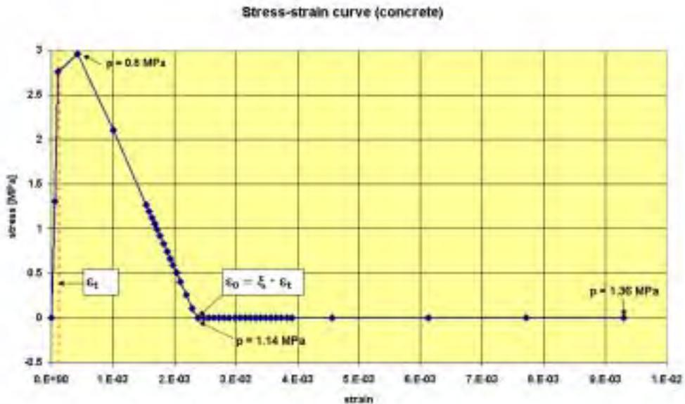
Fig. 21: Part of a typical stress-strain curve for a integration point in concrete, components normal to crack face, slice model, pressure only case
