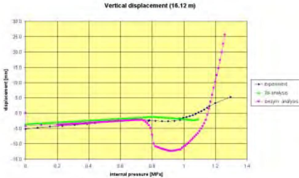
Fig. 13: Vertical displacements at top of the containment (position 16.12 m above basemat), pressure only – experimental values and calculated results
