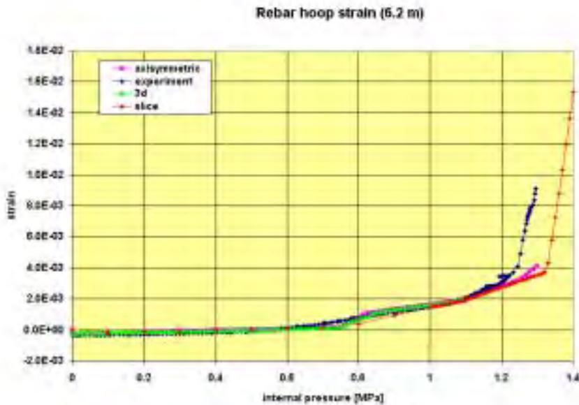
Fig. 14: Hoop rebar strains in the cylindrical part of the containment (position 6.2 m above basemat), pressure only – experimental values and calculated results
