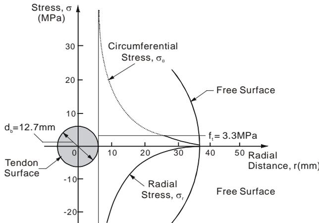
Fig. 4 Transverse stress distributions from isotropic elastic analysis
