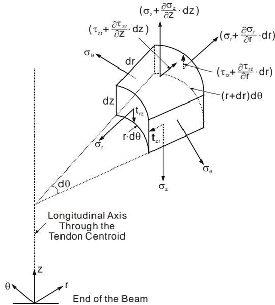
Fig. 2 Three dimensional stresses acting on element
