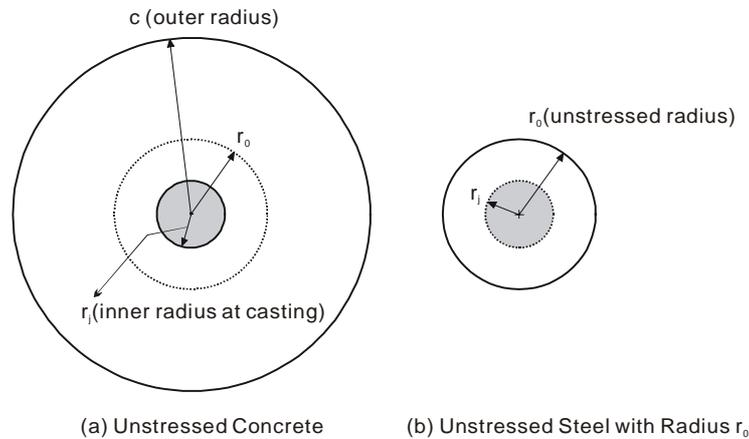
Fig. 1 Physical dimensions of steel and concrete cylinders
