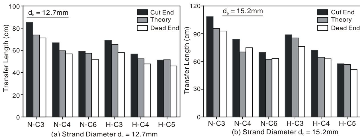
Fig. 15 Comparison of theoretical and experimental transfer length for mono strand test series
