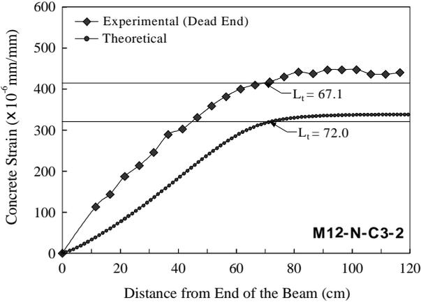
Fig. 8 Comparison of theoretical and experimental strain build-up curves for specimen M12-N-C3-2
