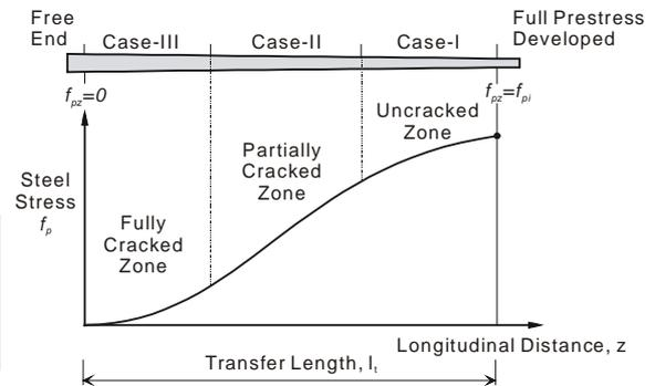
Fig. 6 Typical theoretical prestress build-up curves Fig. 7 Stress build-up in the transfer zone
