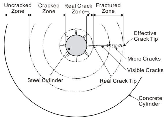
Fig. 5 Nature of cracking around the tendon
