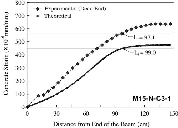
Fig. 9 Comparison of theoretical and experimental strain build-up curves for specimen M15-N-C3-1
