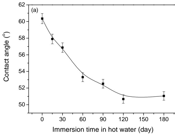
Fig 5. Contact Angle for Immersion Condition.
