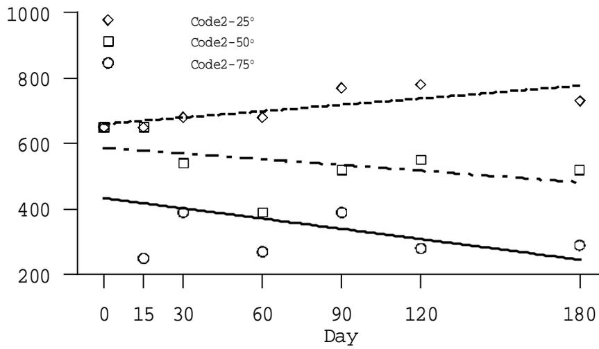
Fig 2. Adhesive Strength of Code 2
