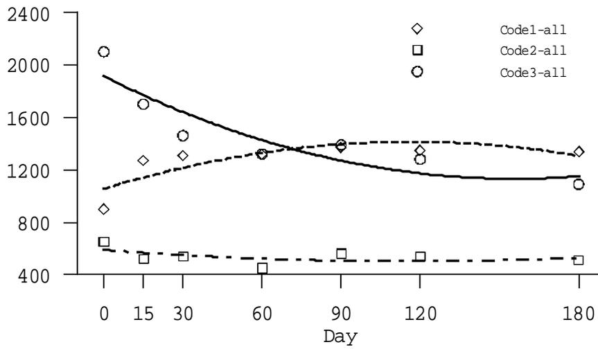
Fig 4. Average Adhesive Strength of Code 1, 2, 3
