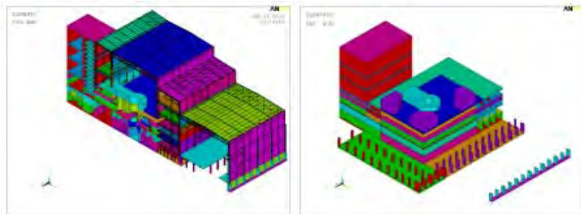
*Fig. 2: The FEM model (longitudinal section, sectional plan under the reactor level – solid finite elements)*
