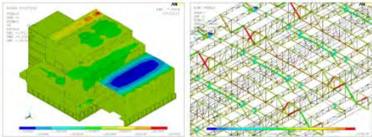
Fig. 7: Examples of combined response – displacements (static and seismic actions)
