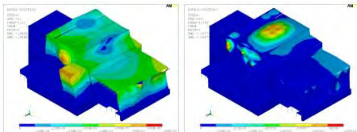
*Fig. 5: Normal modes of vibration (11<sup>th</sup> normal mode –  $f = 3,33$  Hz; normal mode for frequency  $f = 4,49$  Hz)*
