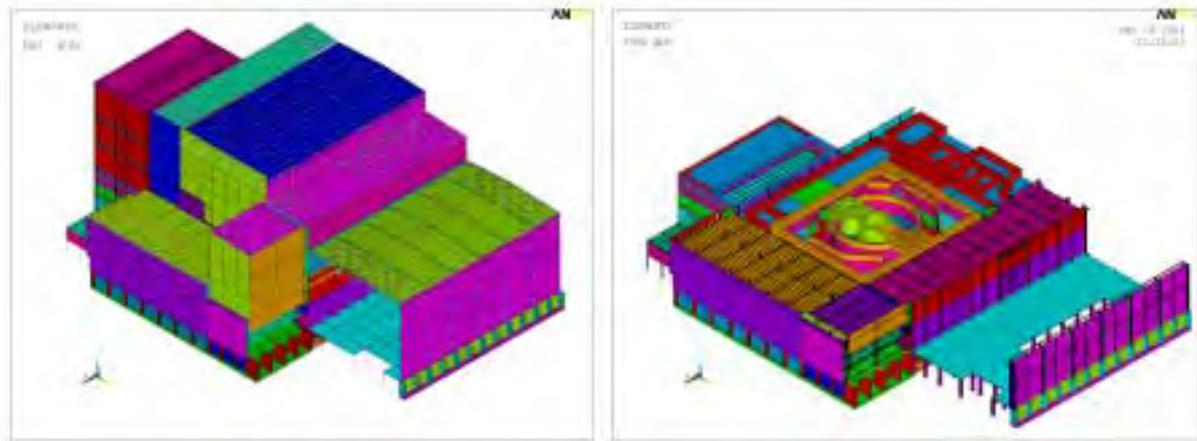
*Fig. 1: The FEM model (general axonometric view, sectional plan on the reactor level)*
