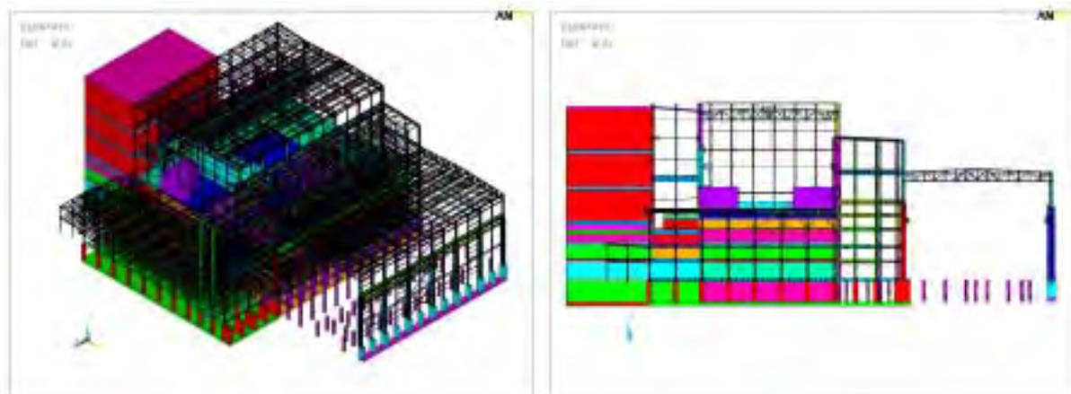
*Fig. 3: FEM model (total view – load bearing structures of facade and roof structure, longitudinal section)*
