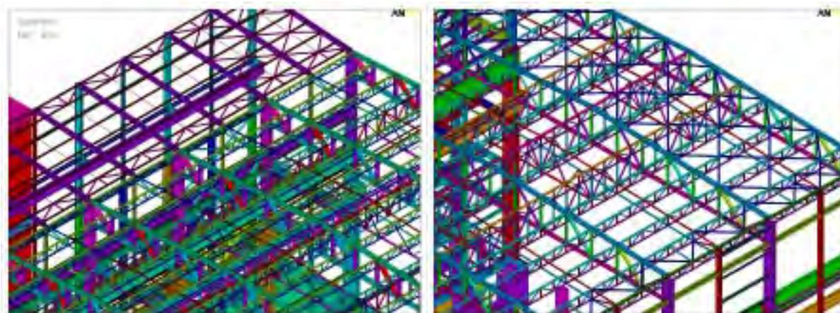
*Fig. 4: Details of the roof structures of the generator and engine room*
