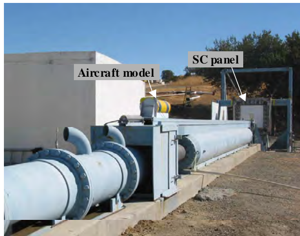
Photo.1 Setting of Aircraft Model and SC Panel on Launcher Facility
