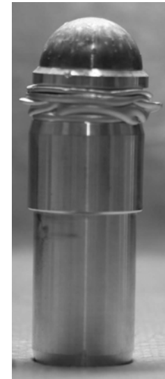
Fig.8 – Condition of deformable projectile after impact
