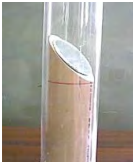
Figure 4 – View of the plexiglas tube with a detail of the mirror inside the tube.
