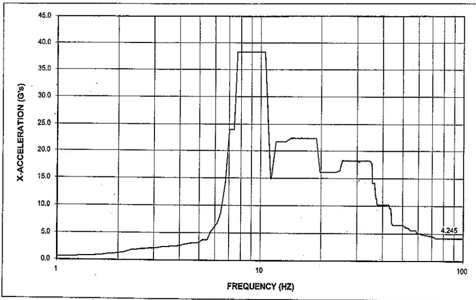
Figure 4: An Example of Required Response Spectra (RRS)
