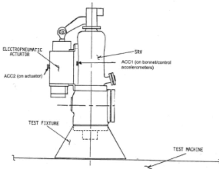
Figure 2: A typical SRV including Actuator mounted on Test Machine for Vibration and Seismic/Dynamic Tests
