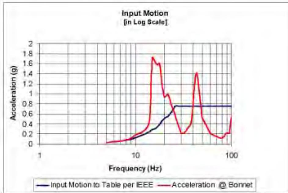
Figure 12: Input Motion to Table and Acceleration at Bonnet
