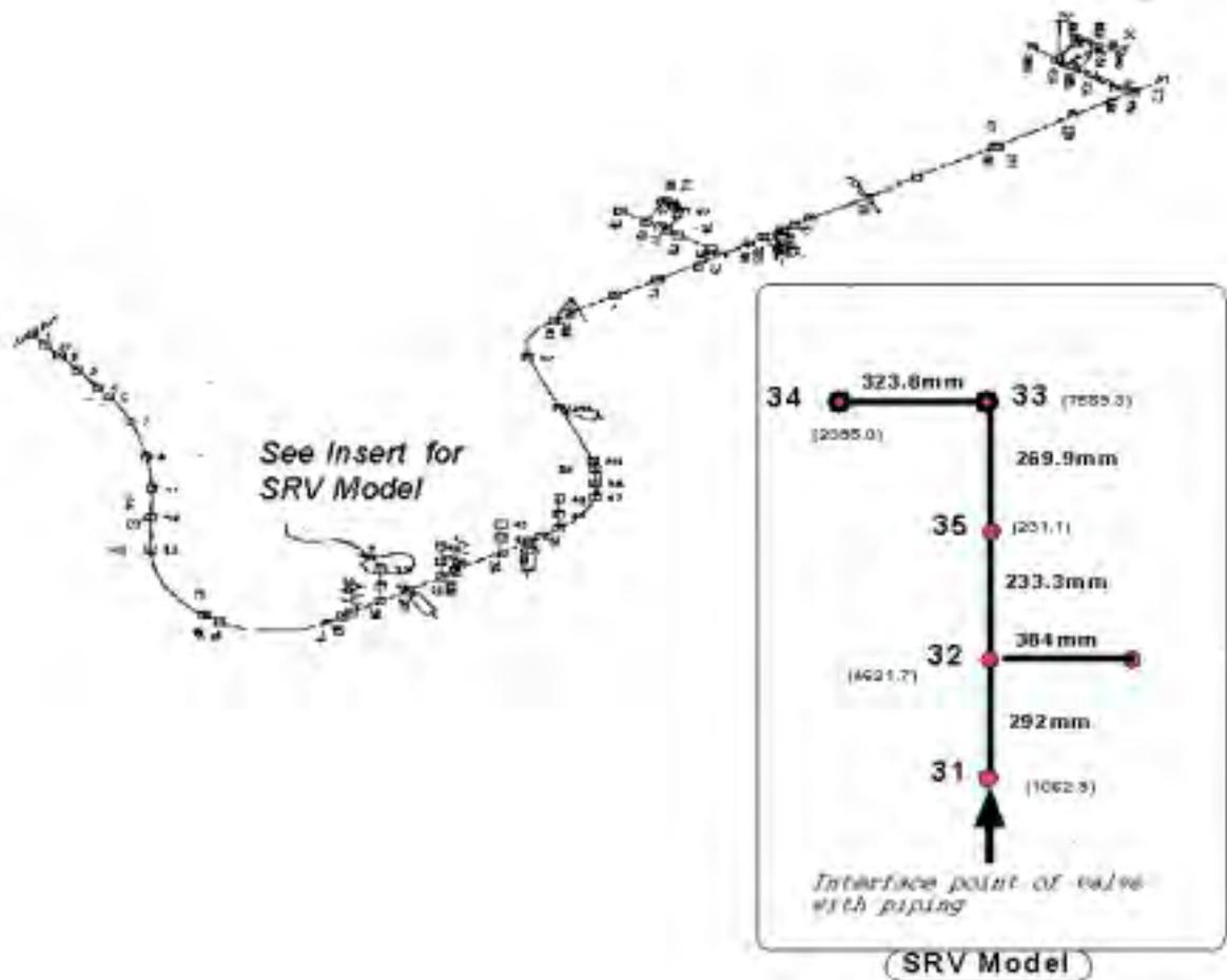
Figure 5: Main Steam Line and SRV Model
