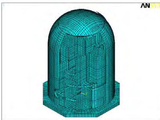
Figure 7: Reactor Building 3D FE Model
