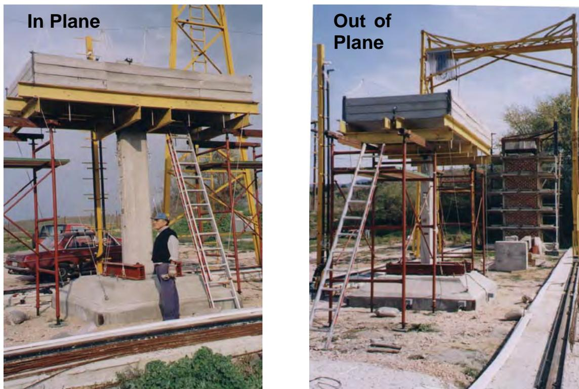
*Figure 7a and b. Erection of the model pier at the Test Site.*
