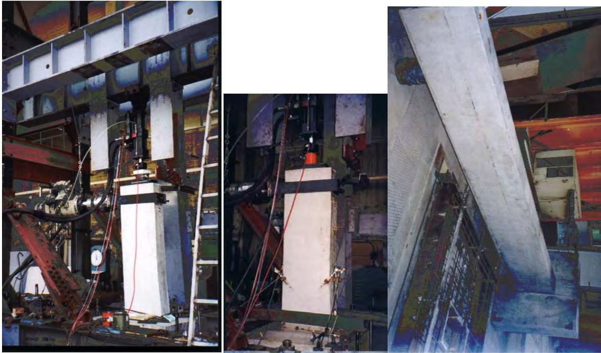
Figure 6. Models A1 and A2 tested at the laboratory and model pier B1 ready for transportation at the Test Site
