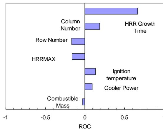
Fig. 11. Sensitivity of the failure time (FA80) to the inputs.
