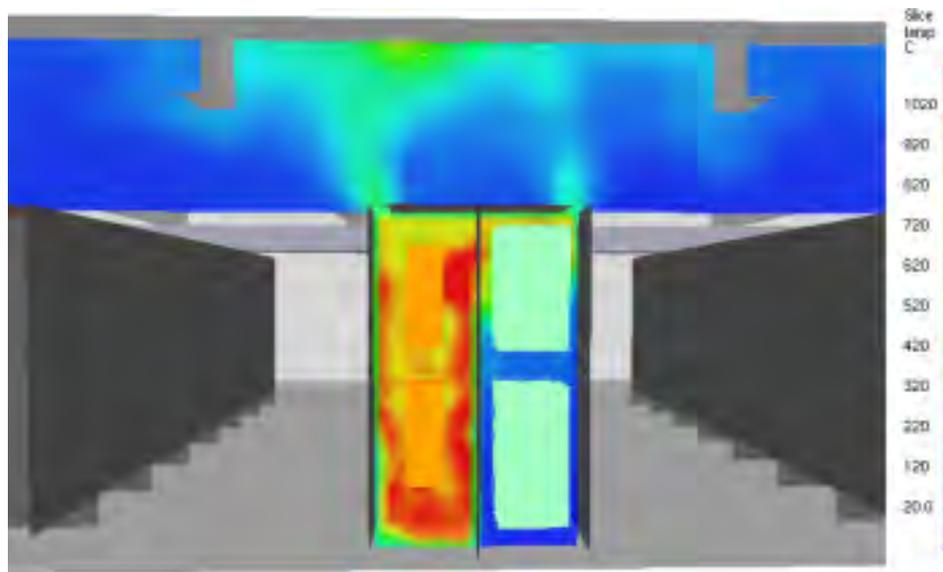
Fig. 9. Instantaneous temperature inside and above the cabinets, 700 s after the ignition.
