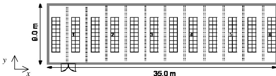
Fig. 6. Plan view of the relay room, with approximate locations of the cabinets and concrete beams. The numbers from 1 to 5 indicate the ignition locations.
