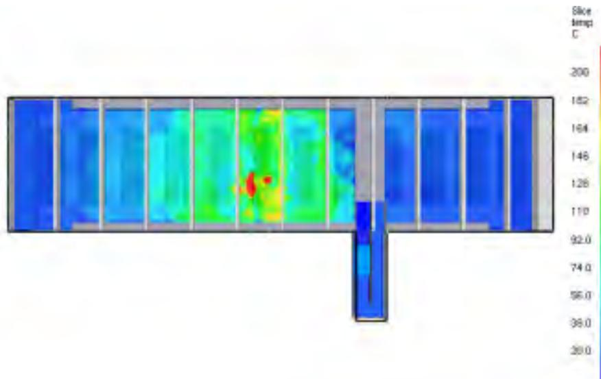
*Fig. 8. Instantaneous temperature at height  $z = 2.4$  m, 700 s after the ignition.*
