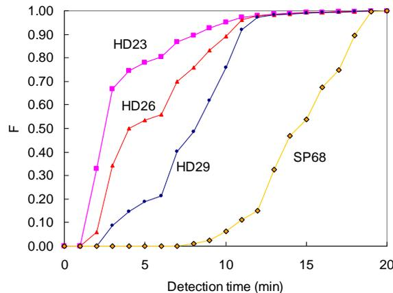
Fig. 12. Cumulative distribution of fire detection times. Curves HD23, HD26 and HD29 correspond to the heat detectors with activation temperatures of 23 °C, 26 °C and °C, respectively. SP68 is a sprinkler head
