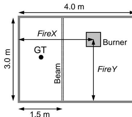
Fig. 1. The geometry of the room fire scenario. GT shows the location of the heat detector and the gas temperature measurement point 5 cm under the ceiling.
