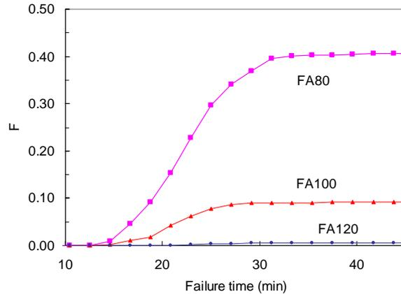
Fig. 10. Cumulative distribution of the target failure times. The three curves correspond to critical temperatures 80, 100 and 120 °C.
