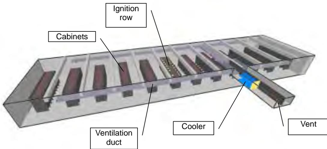
*Fig. 7. An overview of the FDS model of the relay room.*
