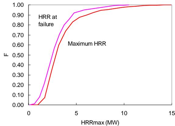
Fig. 14. Cumulative distributions of the heat release rate (HRR) at the time of the failure (FA80) and maximum HRR over the whole fire duration.
