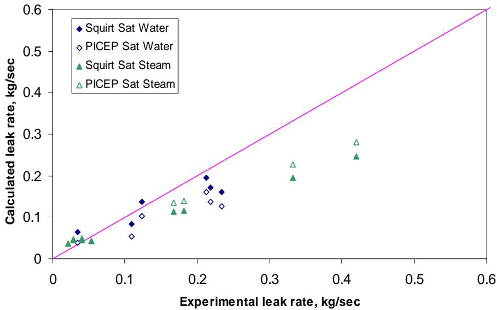
Figure 2. Comparison of PICEP- and SQUIRT-predicted leakage rates with experimentally measured leakage rates from Japanese leakage-rate experiments Matsumoto et al. (1989).
