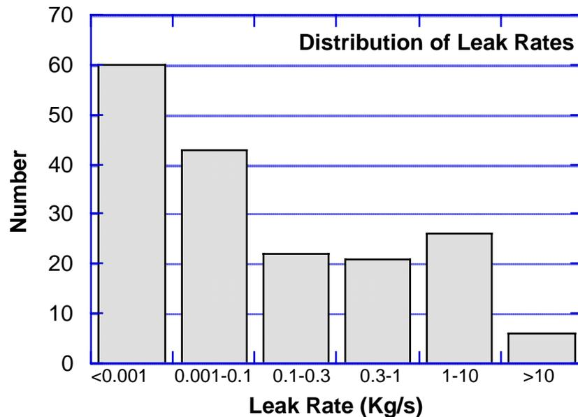
*Figure 7. Distribution of leakage rates by magnitude recorded in the database beginning with 1970. The number of leaks in a given leakage rate range is indicated.*
