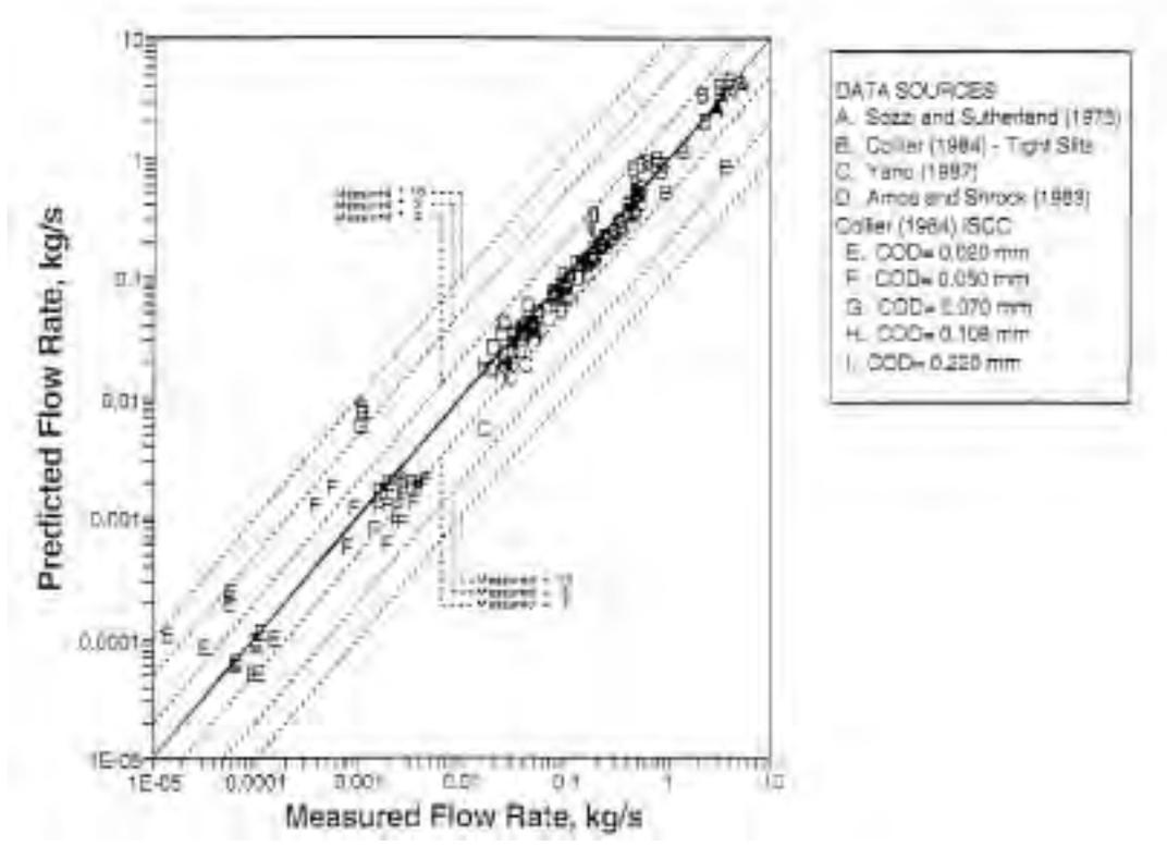
Figure 1. Comparison of two-phase flow leakage rate tests used to validate the initial SQUIRT model.
