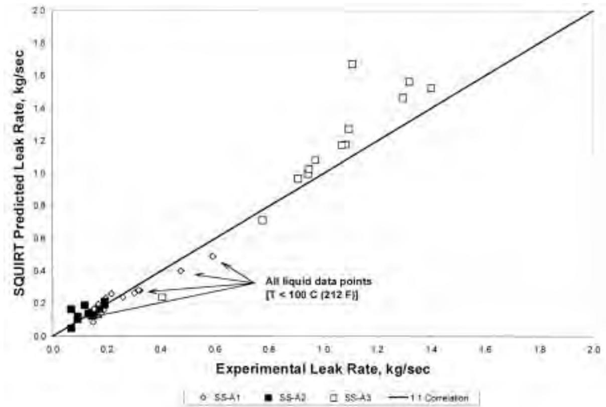
Figure 3. Comparison of SQUIRT-predicted leakage rates versus experimentally measured leakage rates for Ontario-Hydro experiments Boag et al. (1990).
