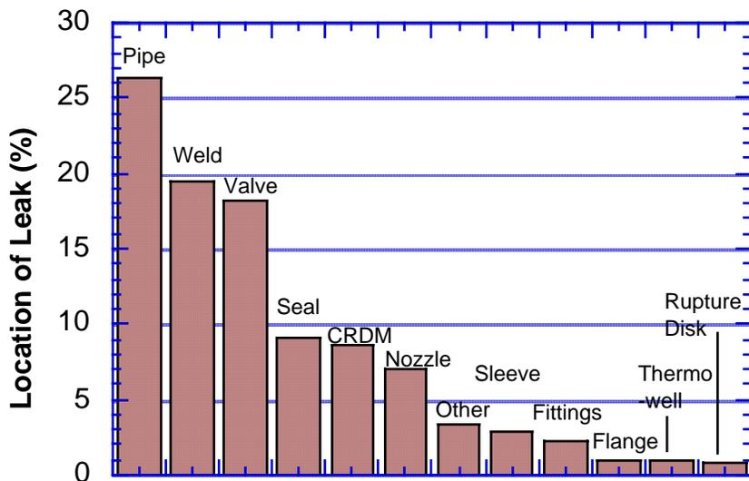
Figure 6. Number of occurrences (percentage) that a location was mentioned in a leak event report. For example, almost 20% of the time the leak involved a weld. About 8% of the leakage events reviewed involved CRDMs, usually detected through visual
