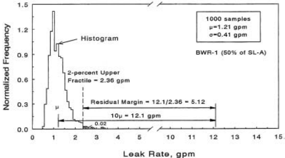
Figure 4. Histogram of leakage rate at 50% Service Level A for case BWR-1 in Rahman et al. (1995) [IGSCC crack case].
