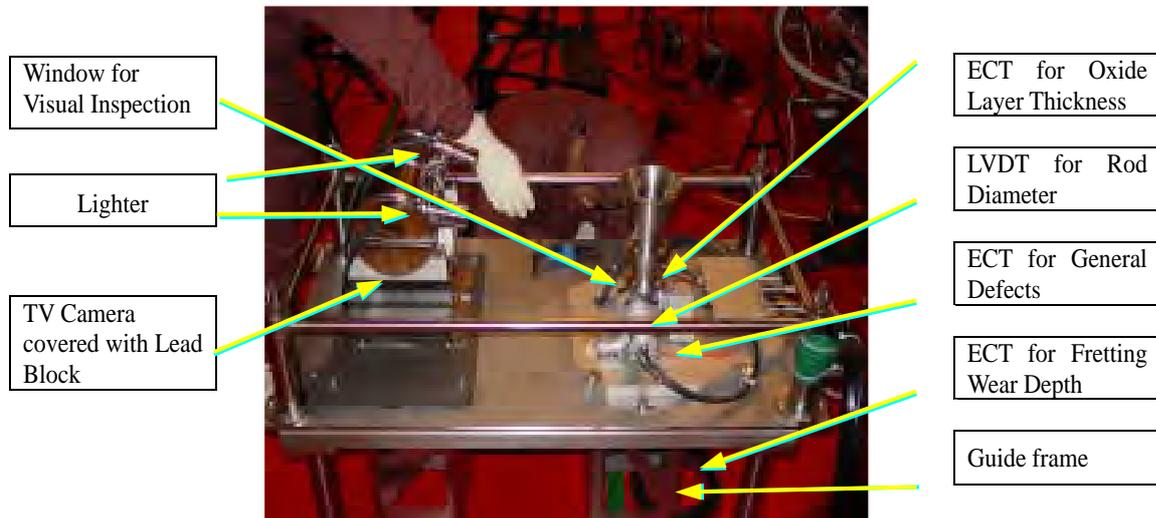
Figure 3. Single Rod Inspection Stand
