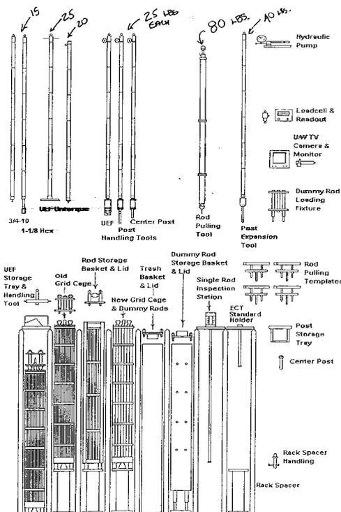
Figure 2. W-CE Type Fuel Repair System
