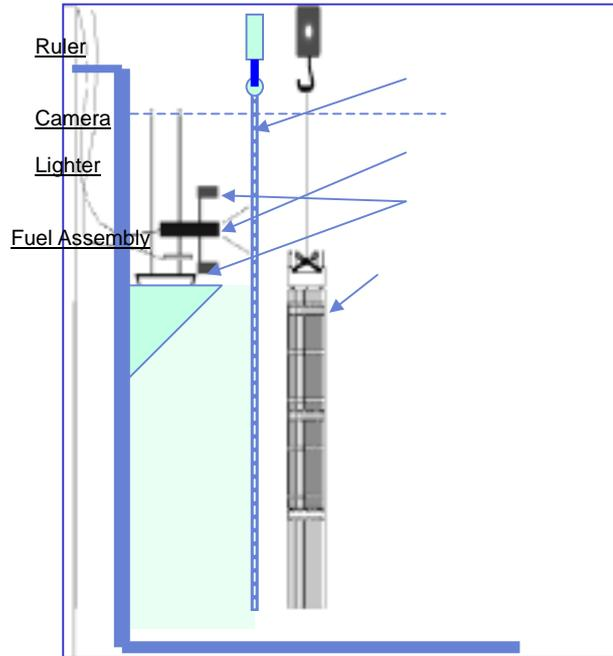
Figure 5. Fuel Assembly Visual Inspection System
