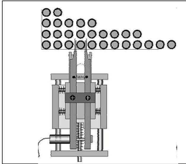
Figure 7. Peripheral Rod Diameter Measurement System
