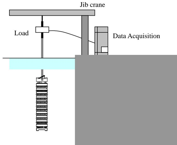
Figure 10. Fuel Rod Dragging Force Measurement System
