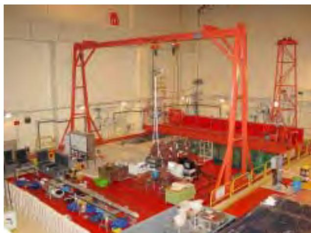
Figure 4. Single Rod Inspection with W-CE Fuel Repair System at YGN#3
