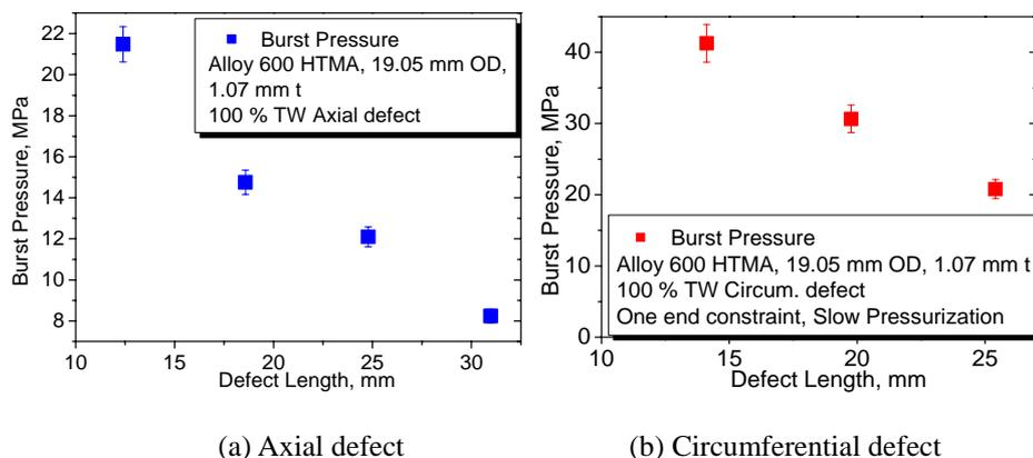
Fig. 5 Comparison of burst pressure of axial and circumferential defect
