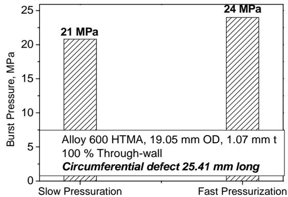
Fig. 6 Effect of the pressurization rate on the burst pressure of circumferential defects
