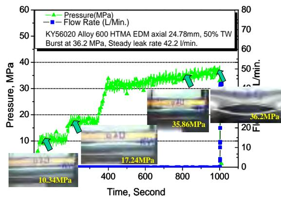
Fig. 1 COD changes of a part through wall axial defect
