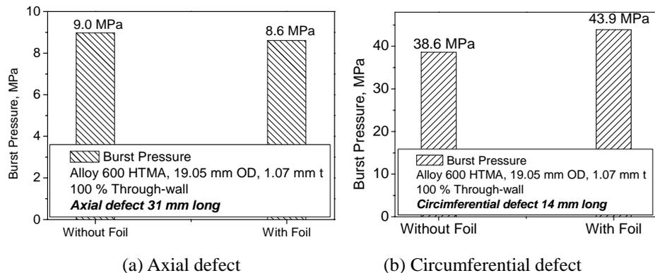
Fig. 7 Effect of back up foil on the burst pressure of axial and circumferential defects
