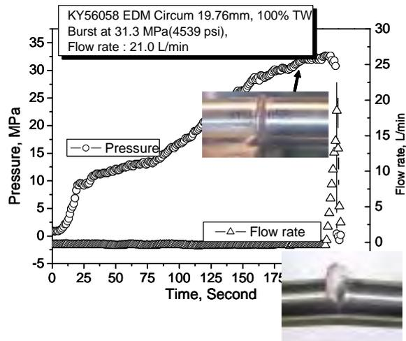
Fig. 3 Crack opening behavior of 100 % TW circumferential defect.
