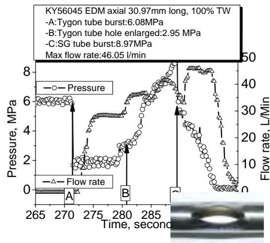
Fig. 2 Crack opening behavior of a 100% TW axial defect.
