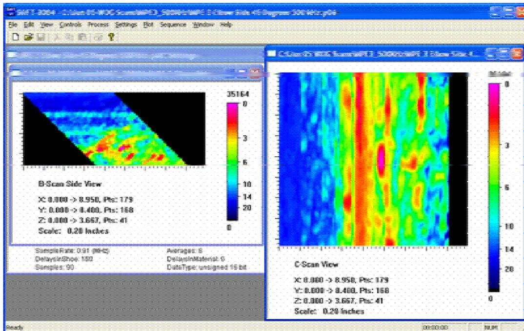
Fig. 3. Composite B-scan (side-view) and C-scan (top-view) views of SAFT processed images resulting from a 500 kHz, 45 degree, L-wave scan of WOG specimen 5.
