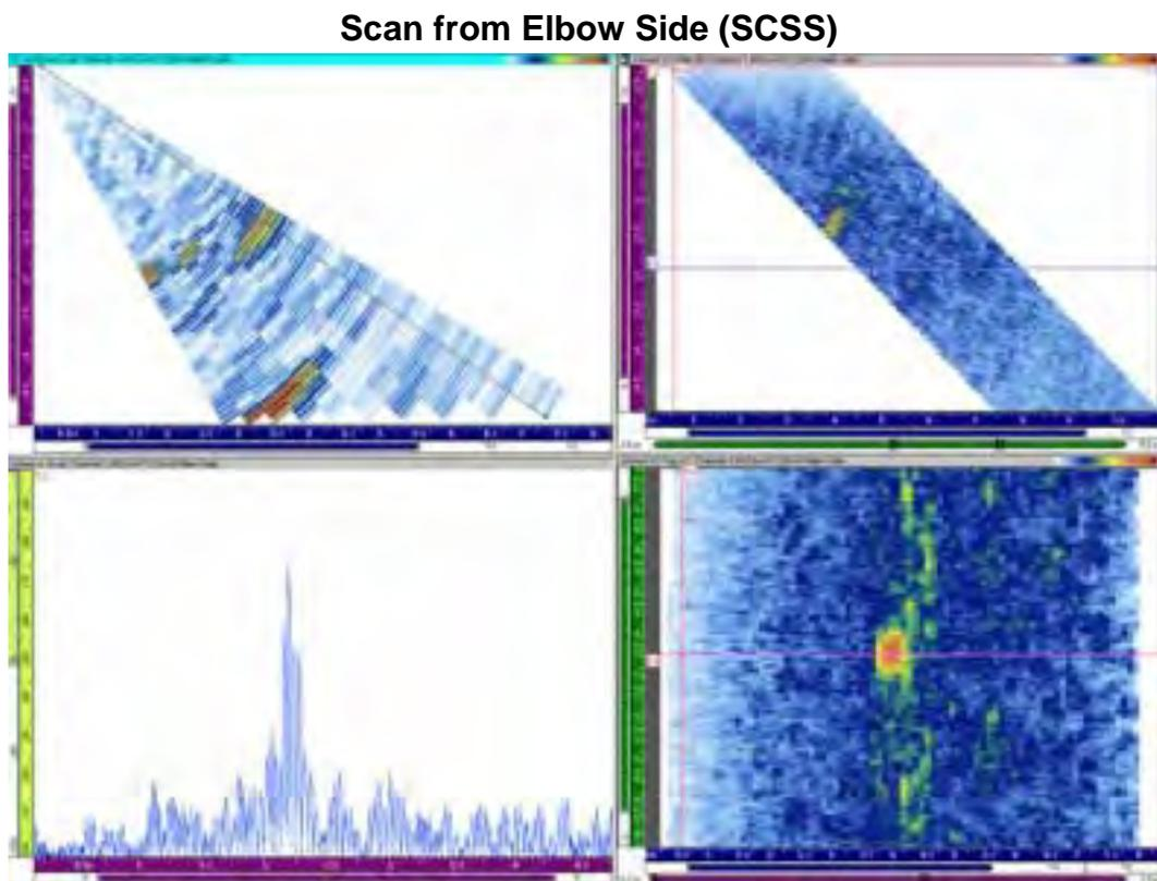
*Fig. 4. PA image illustrating a flaw in a pipe-to-elbow weld imaged using a 1 MHz phased array probe from the statically cast (SCSS), elbow side of the weld. The crack is located on the elbow side of the weld.*
