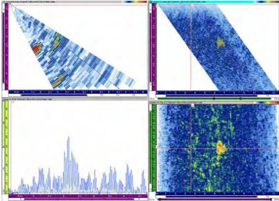
Fig. 5. PA image illustrating the same flaw in figure 4, imaged using a 1 MHz phased array probe from the centrifugally cast (CCSS), pipe side of the weld. The crack is located on the elbow side of the weld.
