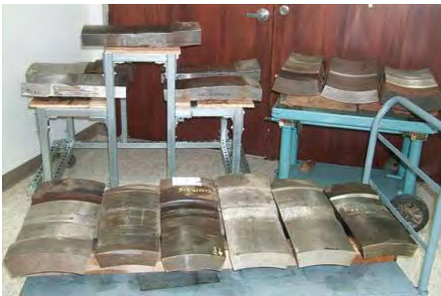
*Fig. 1. Westinghouse Owner's Group sample set of CSS specimens used in this study.*
