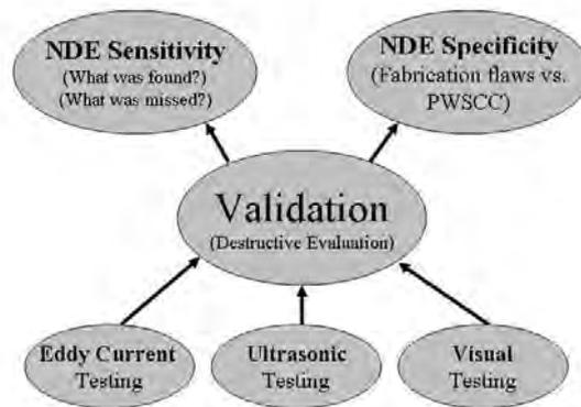
*Fig. 1. NDE Studies of CRDM Nozzle Assemblies removed from service.*
