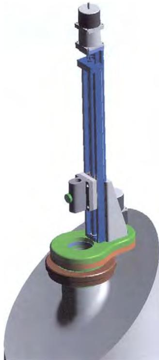
*Fig. 5. Laboratory scanner for inspection from inside the nozzle.*
