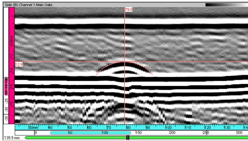
*Fig. 9. TOFD data from the inside of the calibration standard.*
