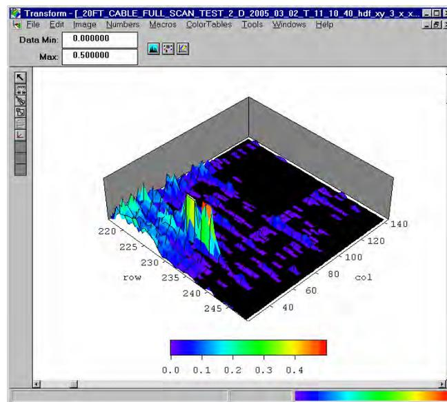
Fig. 6. Eddy Current data from the inside of the calibration standard.
