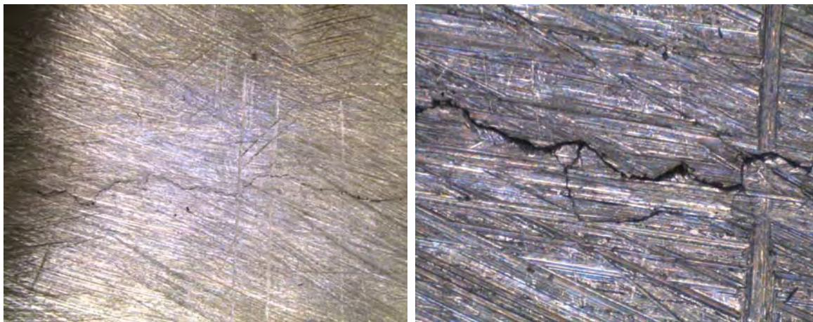
Fig. 10. A 23  $\mu\text{m}$ -wide crack imaged using a Lightwise LW-1.3-S-1394 camera and a diffuse ring light.
