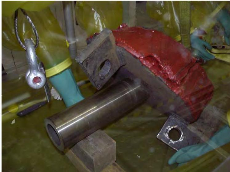
*Fig. 4. CRDM penetration-nozzle assembly in glove box.*
