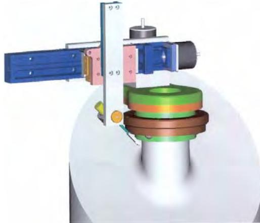
Fig. 7. Laboratory scanner for inspection from surface of the J-groove weld.
