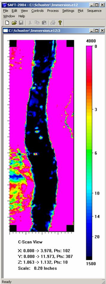
*Fig. 8. Ultrasonic data from inside of a calibration CRDM penetration-nozzle.*
