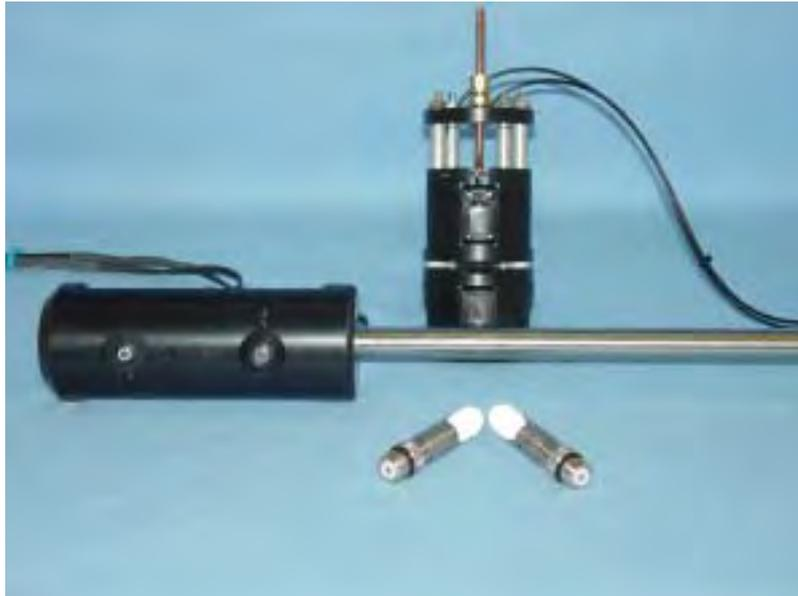
Fig. 5. Ultrasonic focused probes, Eddy Current probe, and TOFD probe for use in inspections from the inside of CRDM penetration tube.
