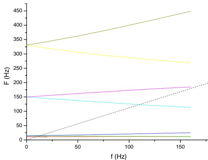
*FIG 2 THE CURVE BETWEEN THE ROTOR SPEED AND NATURAL FREQUENCY*
