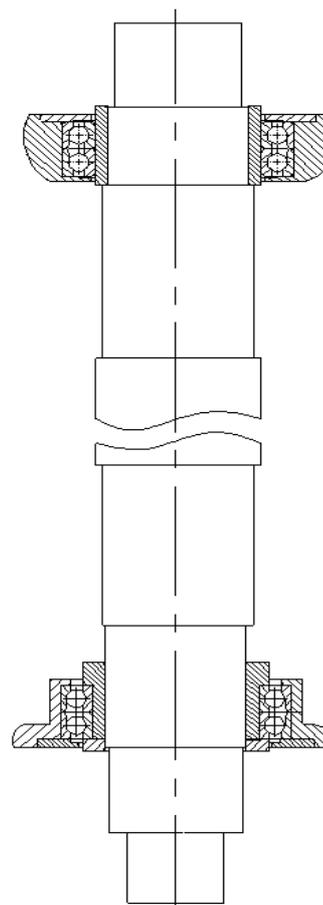
FIG. 1 THE ROTOR STRUCTURE OF BLOWER FAN
