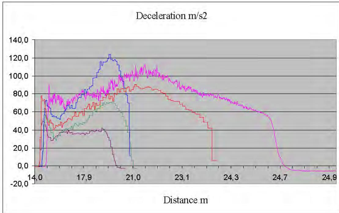
Fig.12 Thickness of LECA layer 20 m, dry shaft, and deceleration as a function of distance.
