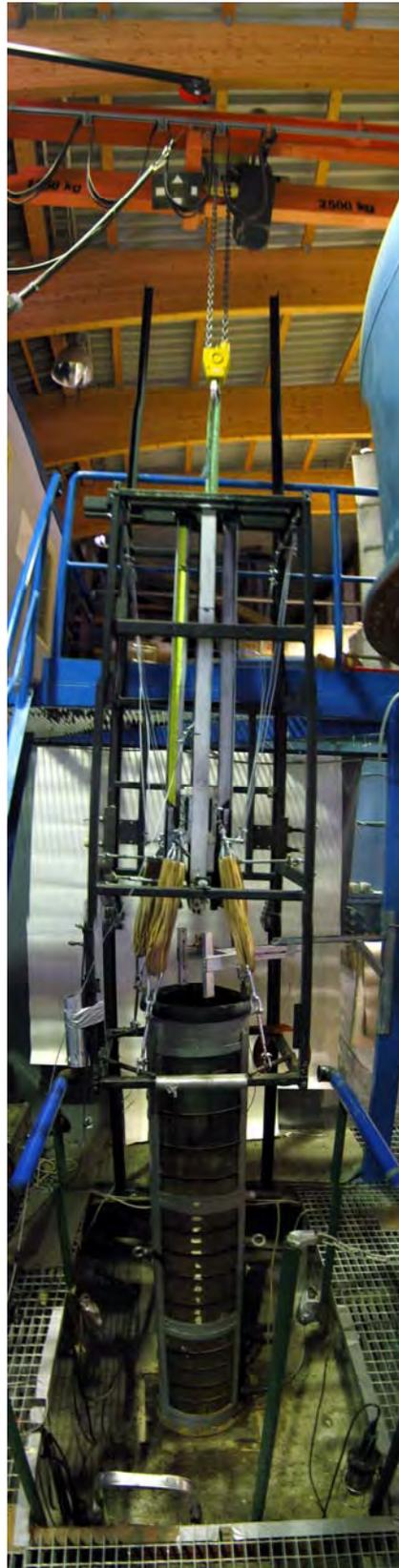
*Fig. 3 Canister sling (right), test piece holder (left upper) and trigger apparatus (left lower).*
