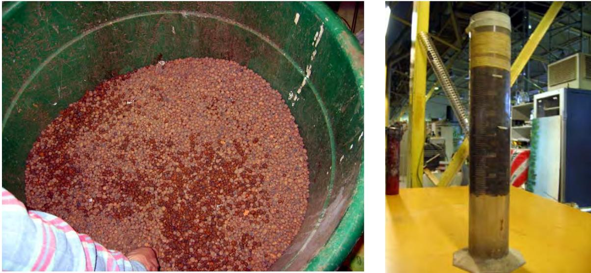
*Fig.10 LECA as a mechanical shock absorber at the shaft bottom. On right water absorbent test of LECA. The water level is halfway of LECA layer at the point of tape.*
