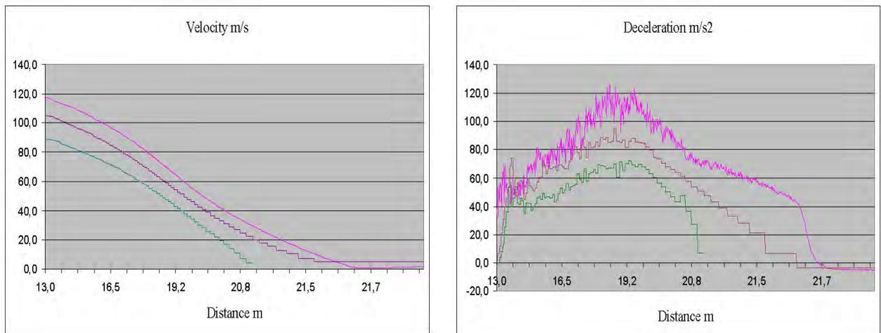
Fig. 3 Wet LECA layer 20 m, 90° nose cone, velocity and deceleration as function of distance.
