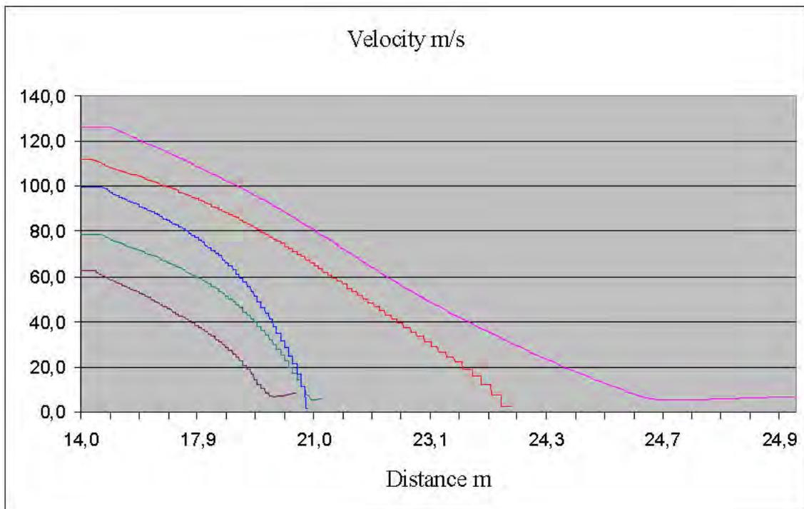
*Fig.11 Thickness of LECA layer 20 m, shaft dry, and velocity as a function of distance.*
