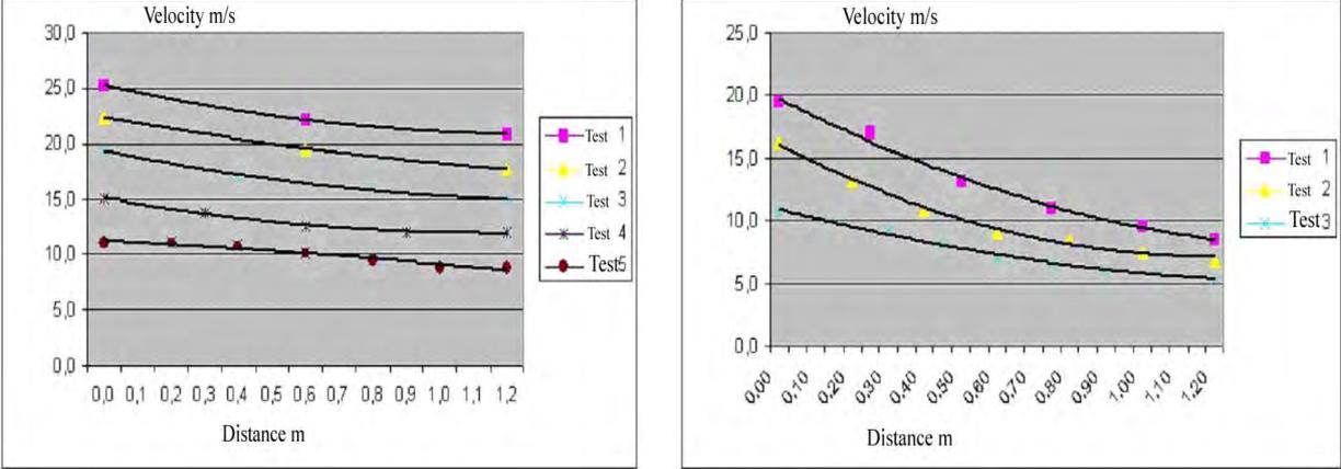
Fig. 6 Velocities as a function of displacement in preliminary test with scale 1:16 (left) and with scale 1:11 (right).
