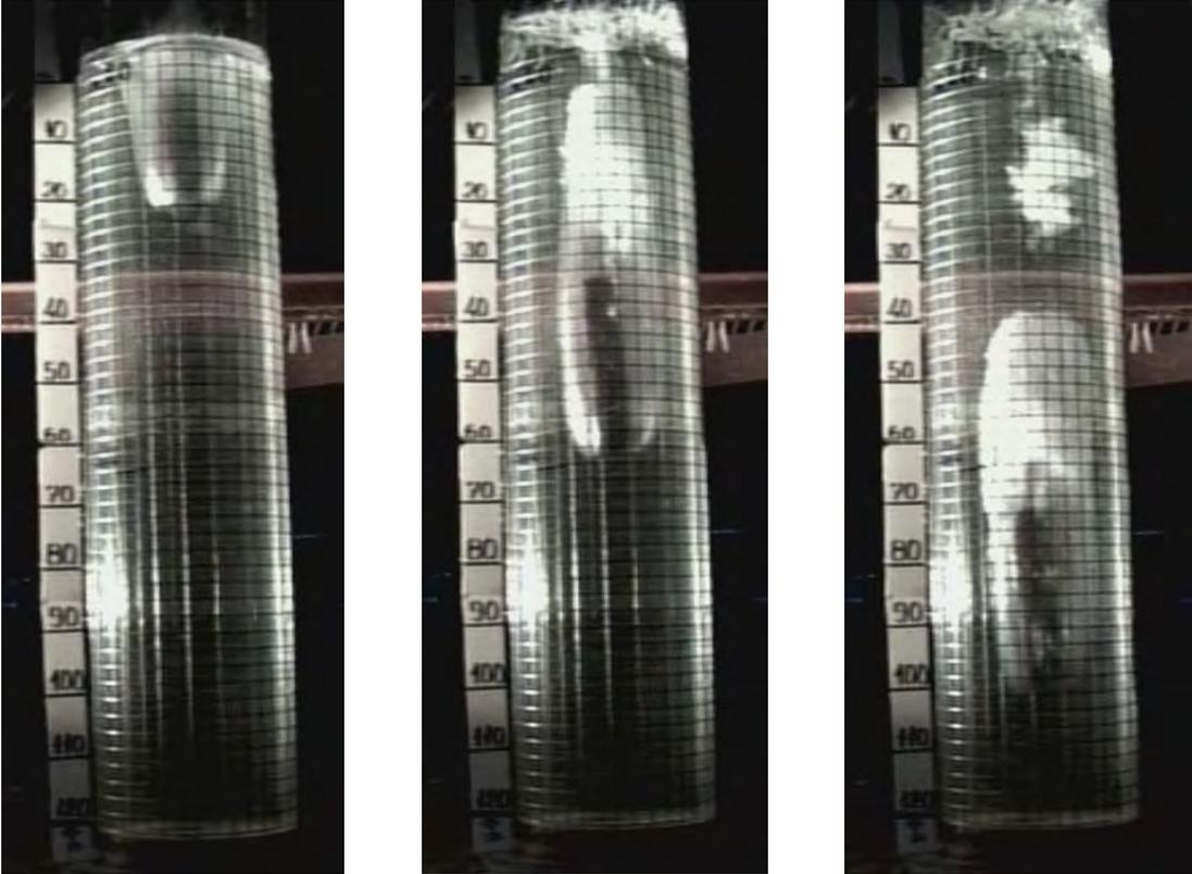
Fig. 7 Test piece entry into water.
