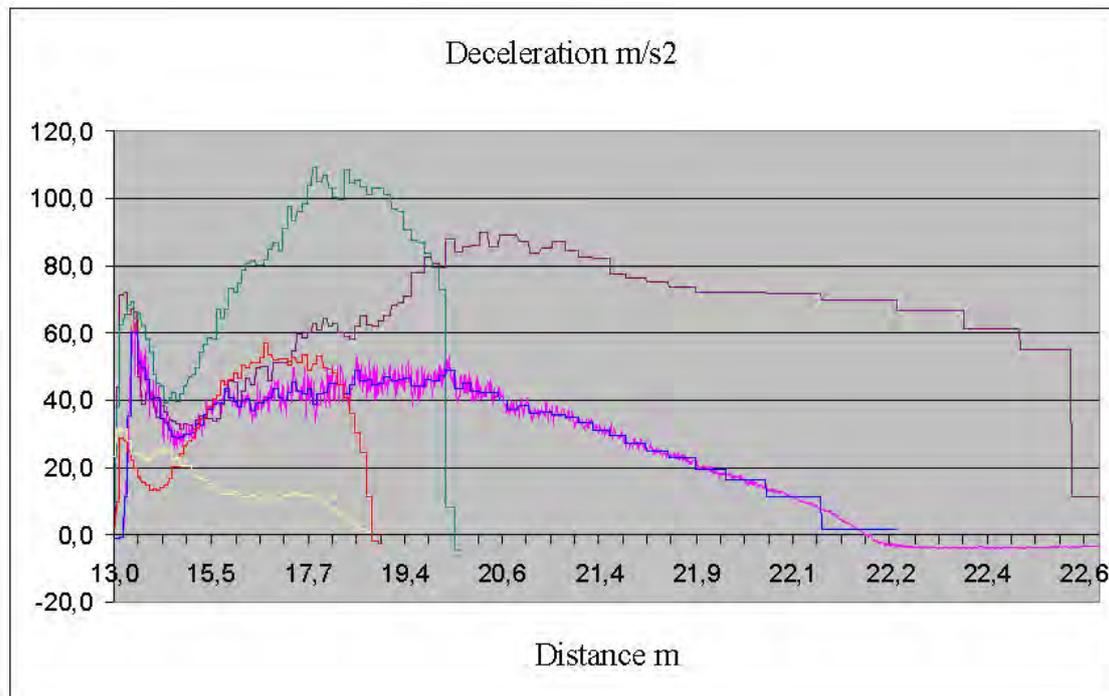
Fig.14 Thickness of LECA layer 20 m, 3 meters water column in shaft, and deceleration as a function of distance.
