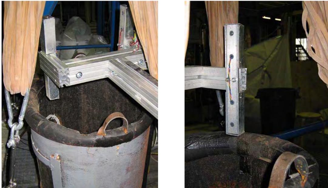
*Fig.4 Velocity measurement gate and photoelectric detector.*
