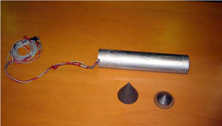
*Fig. 8 Test piece with acceleration sensor. Conical noses used in tests are shown in foreground.*
