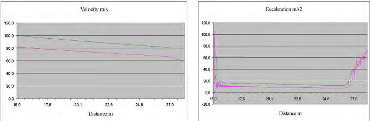
*Fig. 9 Measured velocities and decelerations in water in real scale.*
