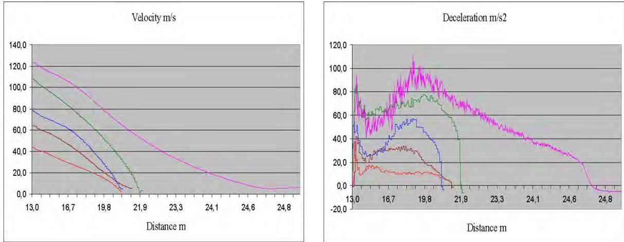
Fig. 2 Wet LECA layer 20 m, velocity and deceleration as function of distance.
