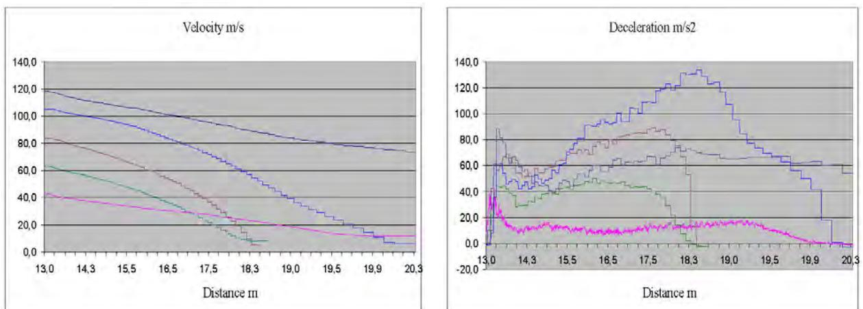
Fig. 1 Thickness of LECA layer 10 m, 10 meters water column in shaft, velocity and deceleration as a function of distance.
