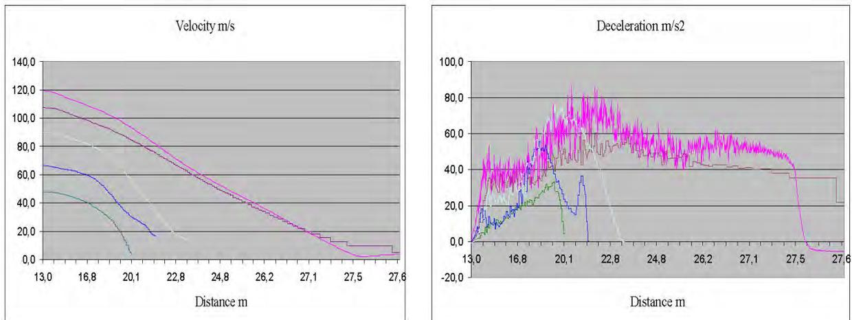
Fig. 4 Wet LECA layer 20 m, 60° nose cone, velocity and deceleration as function of distance.
