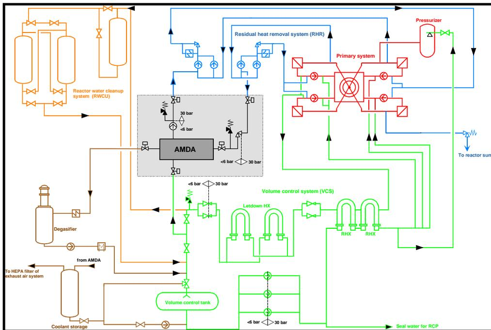
Figure 3: Principle Flow Diagram for FSD at Stade
