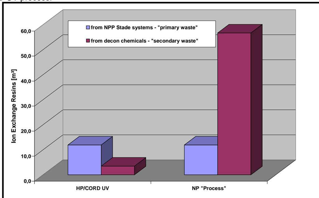
Figure 6: Waste Comparison HP/CORD UV and NP-Processes for FSD Stade
