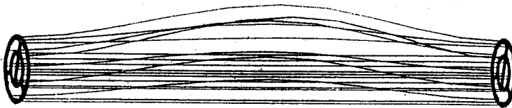
Fig. 6 Buckling of 19 pin fuel bundle
