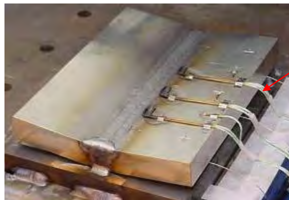
Fig. 1 TIG groove weld plate (3D view)
