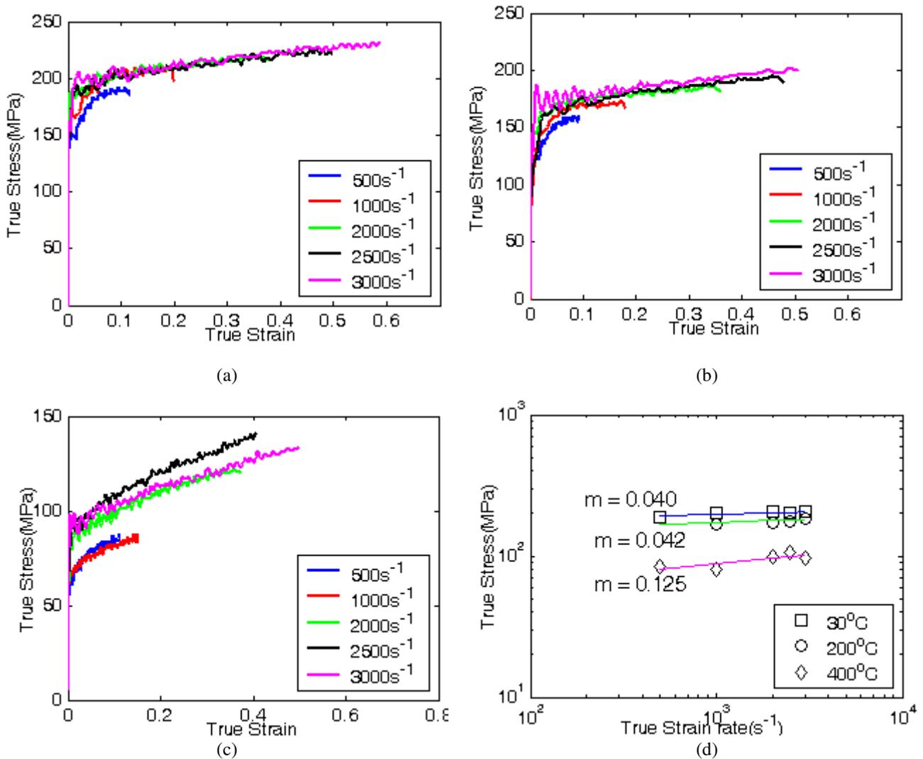
Fig. 2: Stress-strain curve for Al: (a) room temperature, (b) 200°C, (c) 400°C and (d) strain rate sensitivity of Al at 0.1 strain
