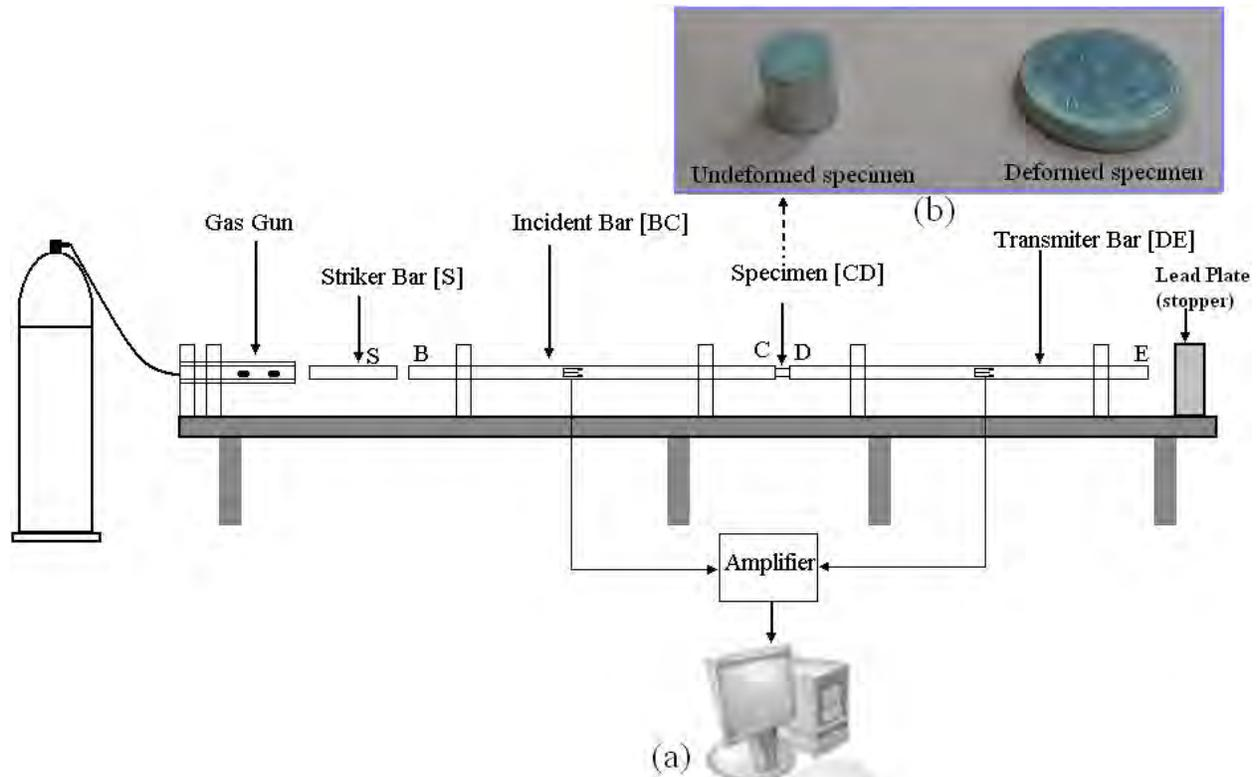
Fig.1: (a) Schematic of Split Hopkinson Pressure Bar and (b) Undeformed & deformed specimen in SHPB test
