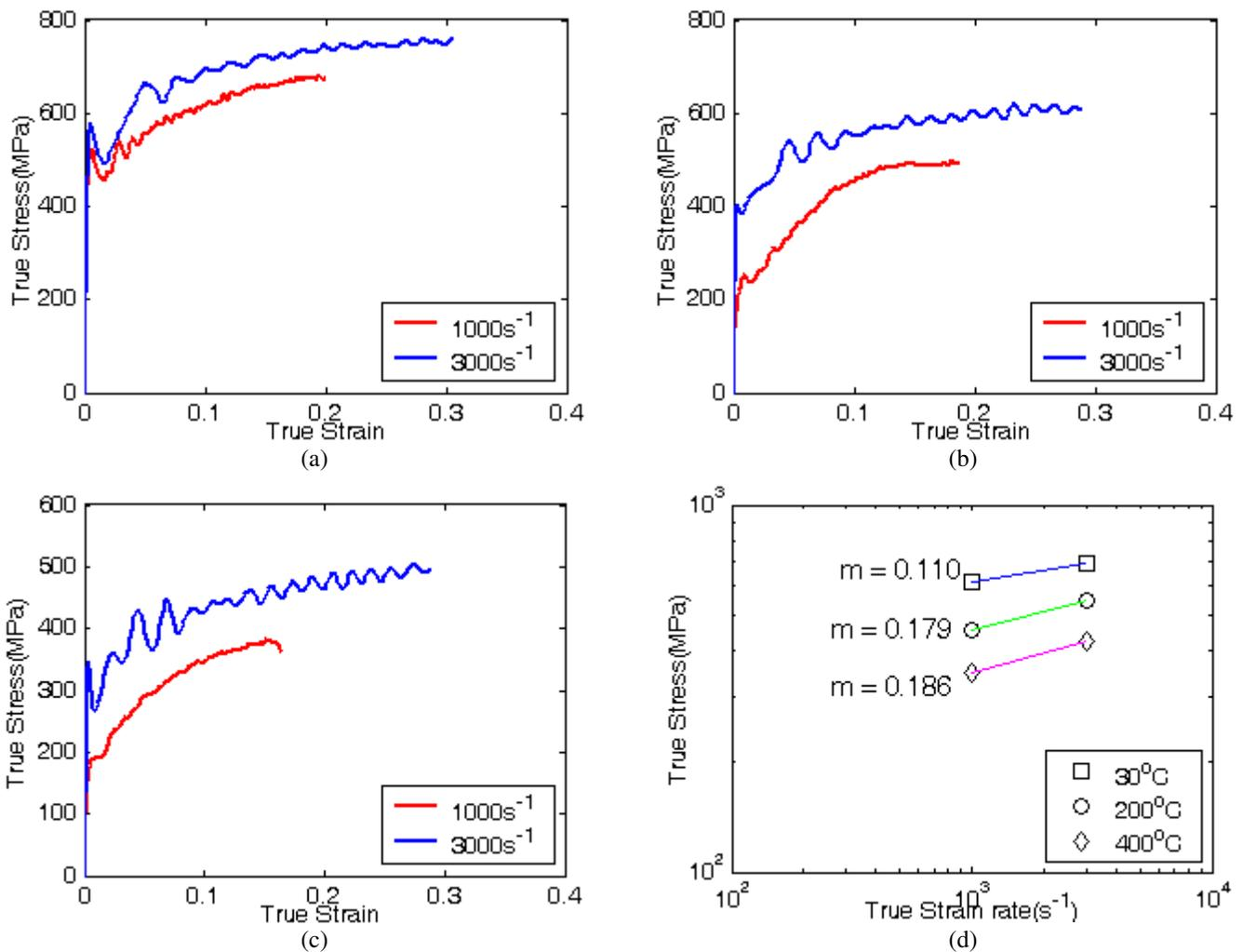
Fig. 3: Stress-strain curve for SA516 Gr.70 steel: (a) room temperature, (b) 200°C, (c) 400°C and (d) strain rate sensitivity of SA516 Gr.70 at 0.1 strain
