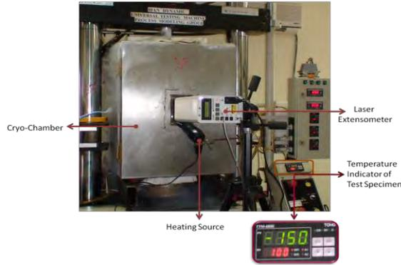
Fig 2a. Basic test facility along with accessories (Exterior view)
