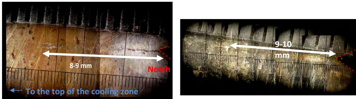
(a) Top crack (after 10000 thermal cycles)
