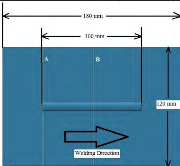
Figure 1: Geometry of Bead on plate
