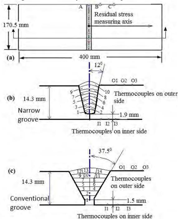
Figure 2: Schematic details for pipe weld joints of (a) Residual stress and temperature measurement for (b) Narrow groove and (c) Conventional V-groove
