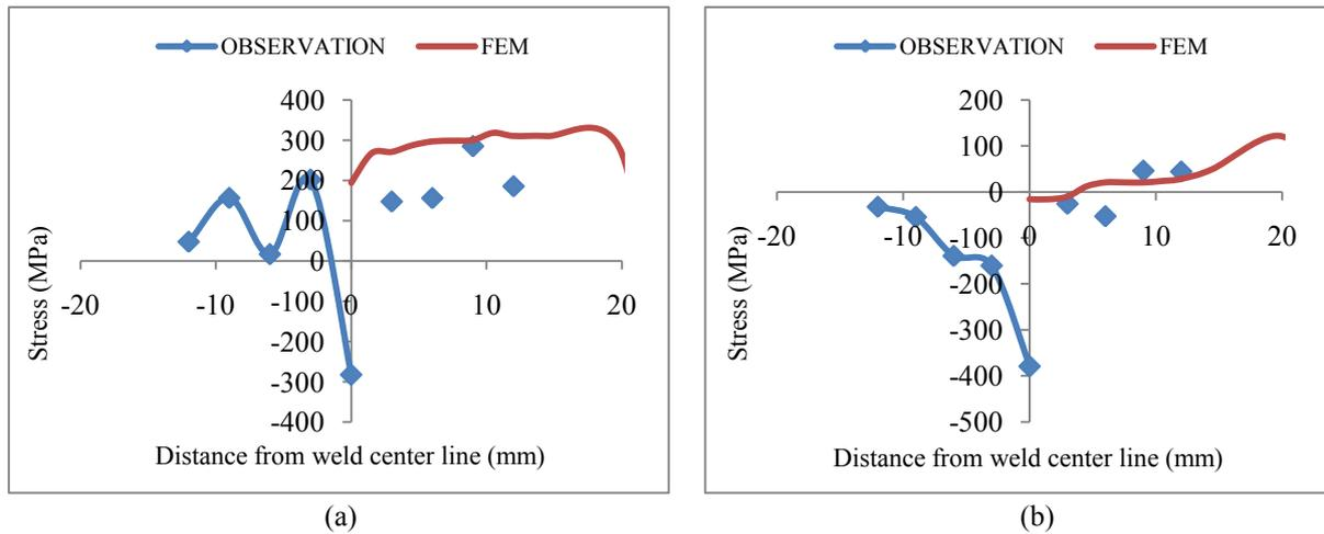
Fig. 7 (a) Longitudinal and (b) Transverse residual stress at middle of bead on plate
