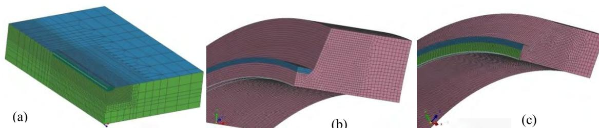
Fig. 3: Finite element model used for thermal analysis in case of: (a) Bead on Plate, (b) Narrow groove GTAW, (c) Conventional groove GTAW
