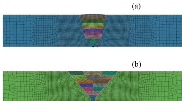
Fig. 5 Two dimensional axy-symmetry finite element model used in mechanical analysis for (a) Narrow groove (b) Conventional V-groove
