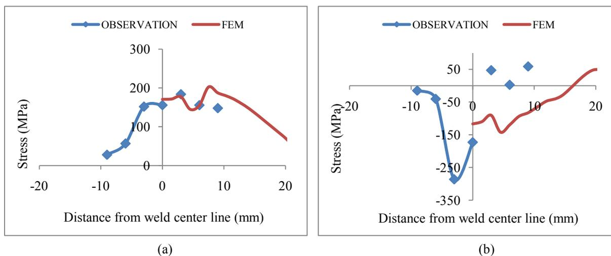
Fig. 6 (a) Longitudinal and (b) Transverse stress at start of bead on plate
