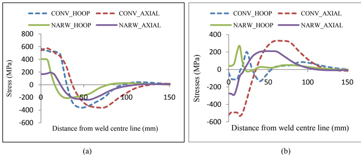
Fig. 10 Residual stress predicted using FEM on (a) inner surface and (b) outer surface
