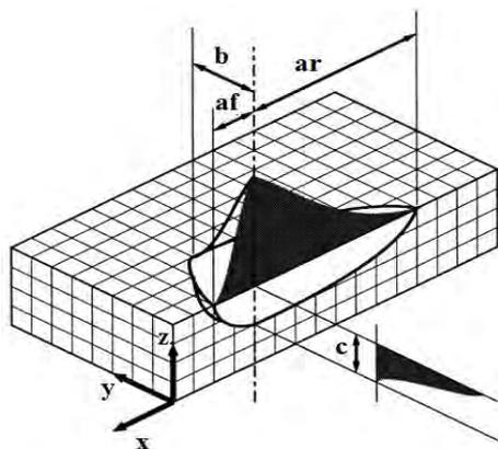
Fig. 4 Double Ellipsoidal Heat Source
