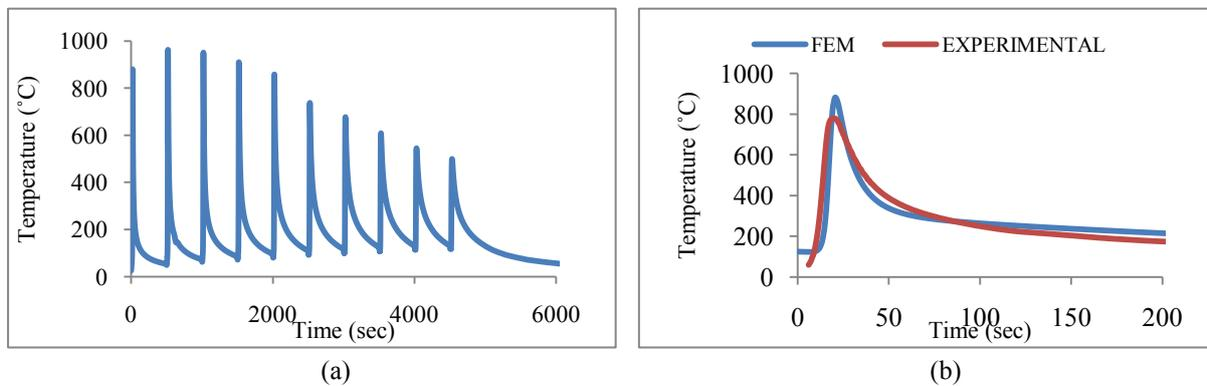
Fig 8 (a) Thermal cycle predicted using FEM analysis (b) Comparison of thermal cycle; at 4mm from weld centerline on inner surface
