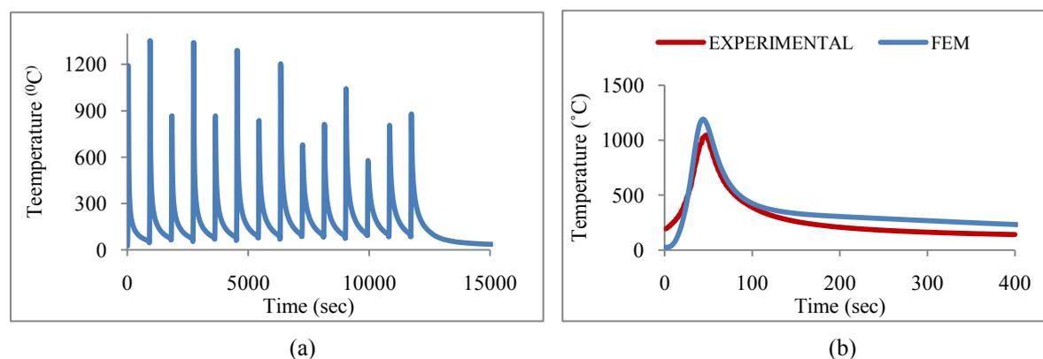
Fig. 9 Thermal cycle at 4 mm from weld centerline on inner surface (a) predicted using FEM (b) comparison using FEM and experimental observation
