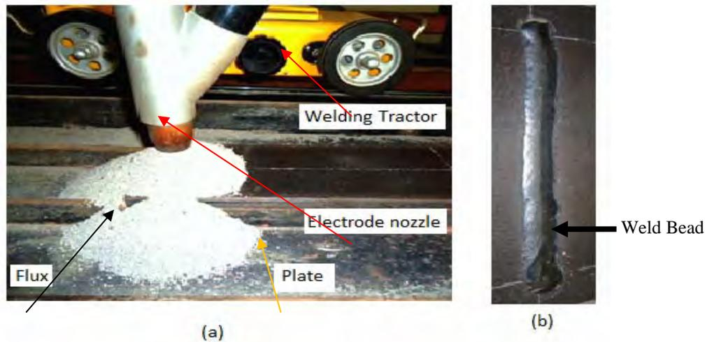
Fig. 1 (a) The SAW setup for experiment and Fig. (b) The butt-bead-on plate
