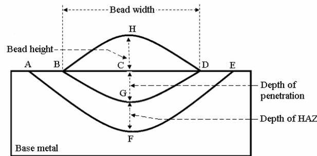
Fig. 2 Schematic of SAW weldment shape profile
