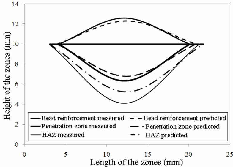
Fig. 3 SAW weldment shape profile of test case NO. 3 (Table 7)
