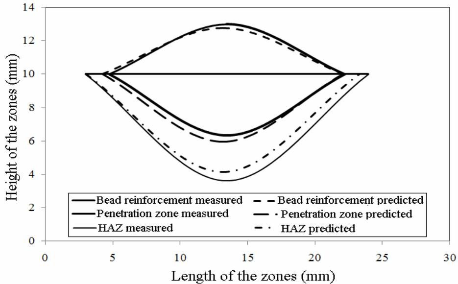
Fig. 4 SAW weldment shape profile of test case NO. 5 (Table 7)
