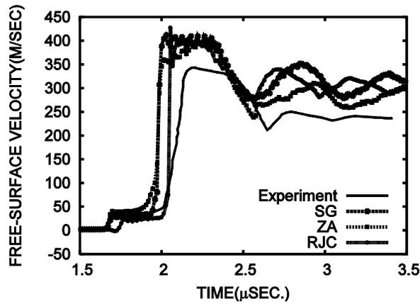
Fig.2: Experimental and computed free-surface velocity profiles for experiment labeled B-16 using SG, ZA and RJC models, with a mild steel target.
