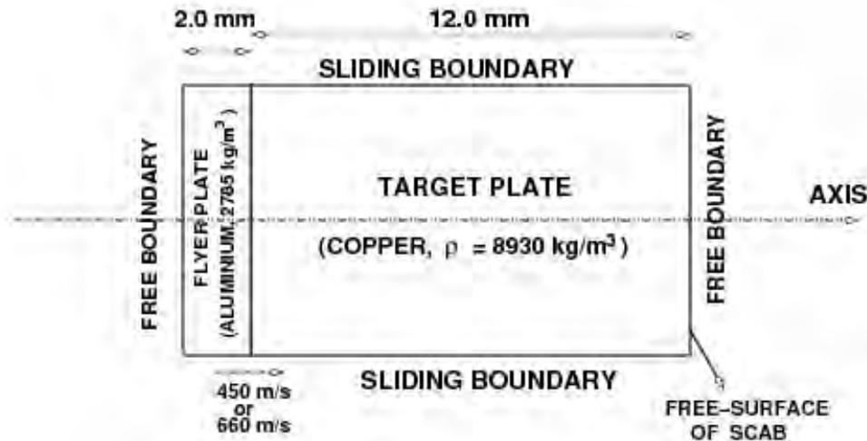
Fig.1: Schematic of the computational mesh for 1-D simulation (not to scale). Boundary conditions are also specified. The thicknesses of both plates are greatly exaggerated.
