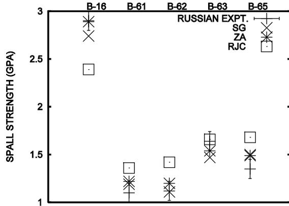
Fig.6: Computed spall strength values for various experiments
