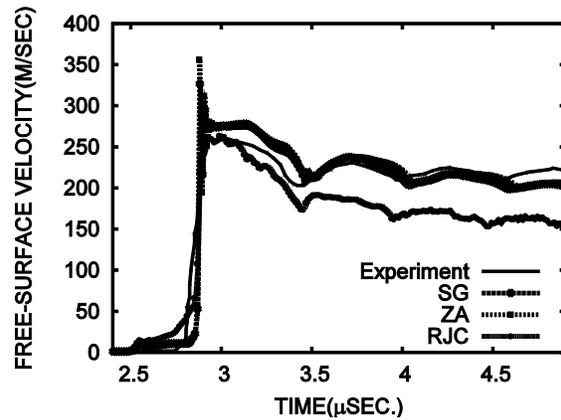
Fig.3: Experimental and computed free-surface velocity profiles for experiment labeled B-62 using SG, ZA and RJC models, with a copper target.
