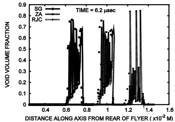
Fig.5: Normalized void volume computed in copper for experiment labeled B-62, using SG, ZA and RJC models. The curves corresponding to different models have been displaced for clarity; otherwise, void growth occurs in the same region with all models.
