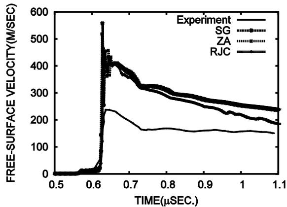
Fig.4: E experimental and computed free-surface velocity profiles for experiment labeled B-65 using SG, ZA and RJC models, with a copper target.
