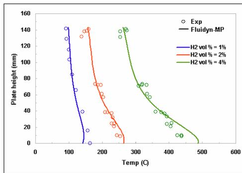
Fig. 10: Catalytic plate temperature profile with different concentrations of H<sub>2</sub>
