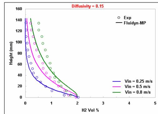
Fig. 13: Concentration profile for different flow rates
