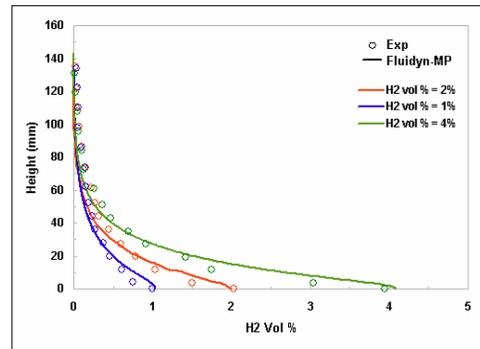
Fig. 11: Hydrogen concentration profile with different concentrations of H<sub>2</sub>
