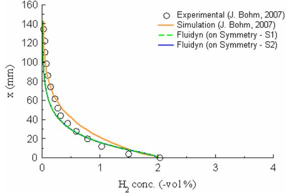
Fig. 7: Hydrogen concentration profile
